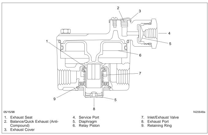
Fig. 4, R-14 Relay Valve (sectional view)
