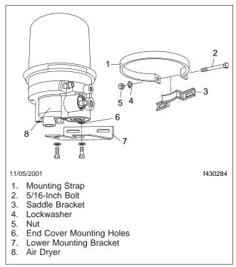
Fig. 1, Bendix AD-IP Air Dryer
