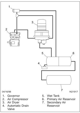
Fig. 1, Air Dryer Air Plumbing Diagram
