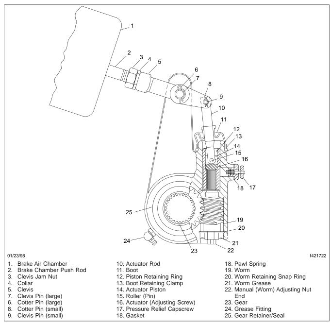
Fig. 2, Automatic Slack Adjuster (sectional view)
