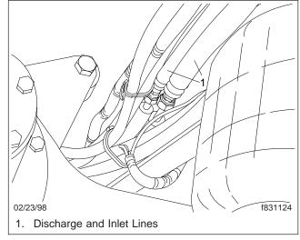
Fig. 2, Discharge and Inlet Lines
