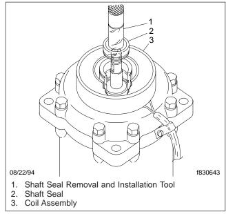
Fig. 2, Remove the Shaft Seal
