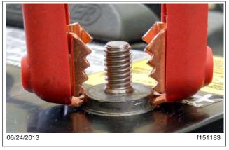
Fig. 1, Tester Clamps Attached to the Post
