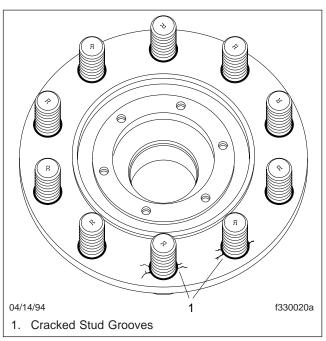
Fig. 2, Damaged Front Axle Wheel Hub
