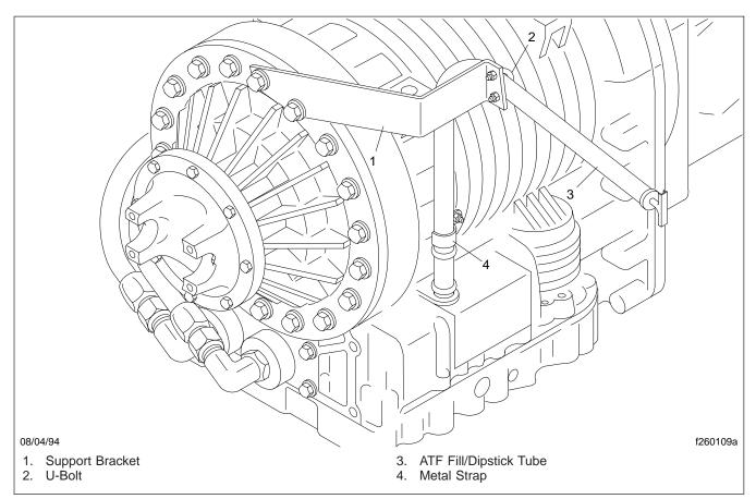
Fig. 4, Removing the Fill/Dipstick Tube
