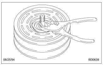
Fig. 8, Install the Shaft Key
