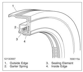
Fig. 2, Wheel Oil Seal Parts
