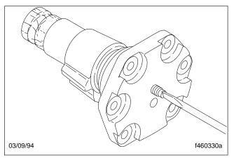
Fig. 10, Screw the Sector Shaft Adjusting Screw into the Side Cover
