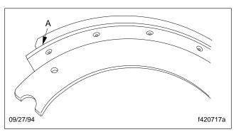
Fig. 5, Area of Feeler Gauge Clearance
