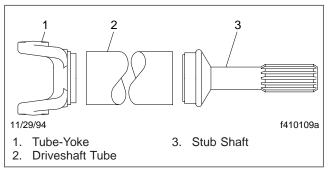
Fig. 17, Driveshaft Tube, Stub Shaft, and Tube-Yoke
