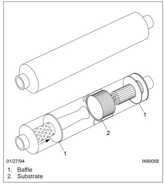
Fig. 2, Typical Catalytic Converter Muffler
