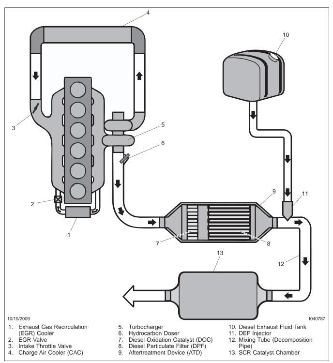
Fig. 1, Aftertreatment System (typical)
