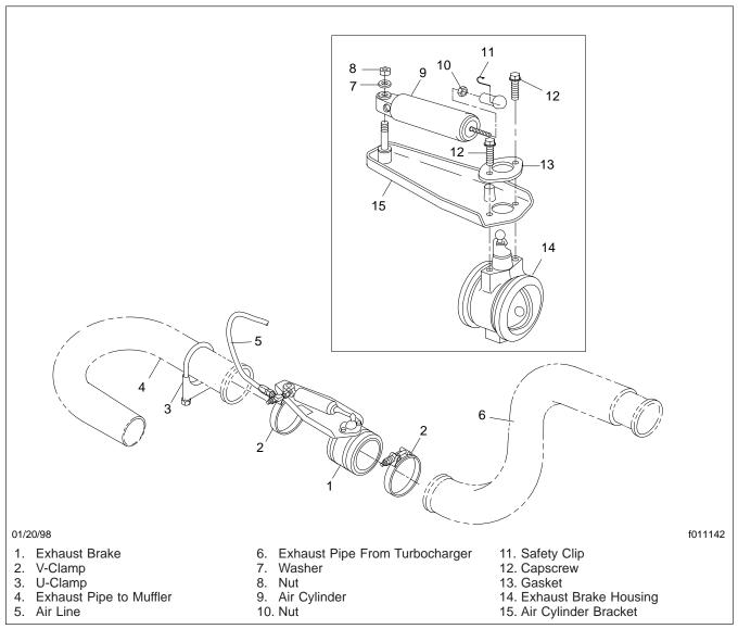
Fig. 1, Jacobs Exhaust Brake
