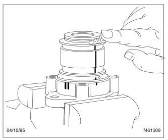
Fig. 34, Greasing the O-Rings
