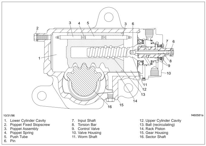
Fig. 2, Steering Gear Sectional View
