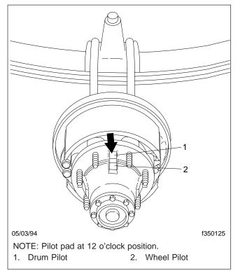
Fig. 3, Front Axle Drum and Wheel Pilots (rear axle similar)
