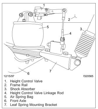
Fig. 1, Typical Front Spring Assembly
