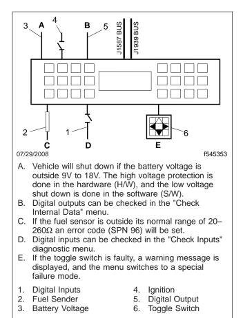
Fig. 2, Possible LBCU Errors
