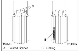
Fig. 10, Damaged Slip-Joint Splines
