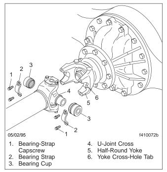
Fig. 4, Coupling of a Spicer or Meritor U-Joint With a Half-Round End-Yoke
