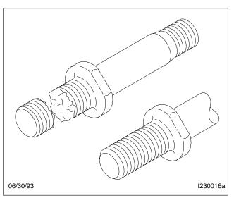
Fig. 5, Damaged Wheel Studs (shouldered type)
