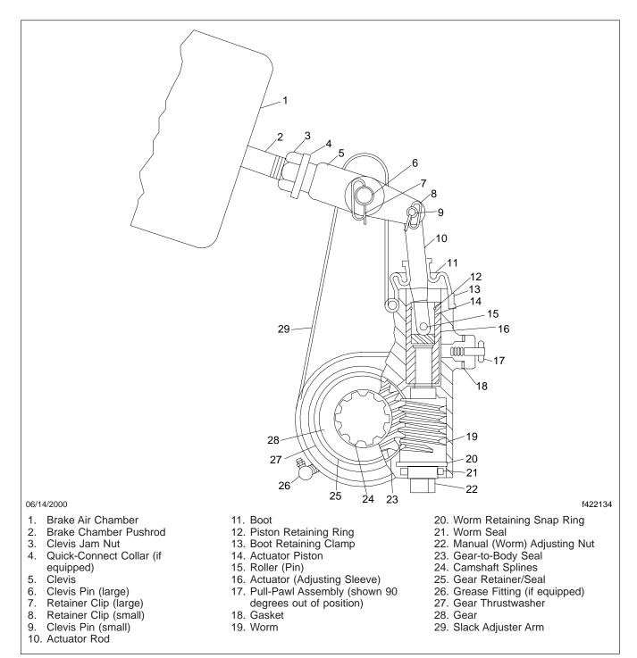
Fig. 1, Automatic Slack Adjuster (sectional view)
