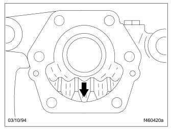
Fig. 94, Check the Tooth Position
