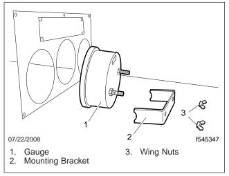
Fig. 1, Wing Nut Mounted Gauge
