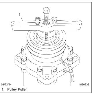
Fig. 5, Position the Pulley Puller Jaws
