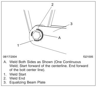
Fig. 3, Alignment Block Welded in Place
