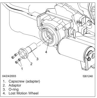
Fig. 4, Adaptor (type A) and Lost Motion Wheel
