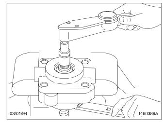
Fig. 63, Check the Torque
