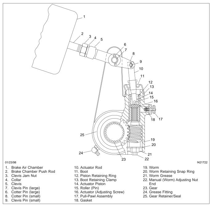
Fig. 2, Automatic Slack Adjuster (sectional view)
