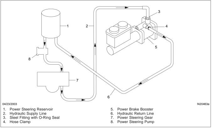
Fig. 1, Power Brake Booster System
