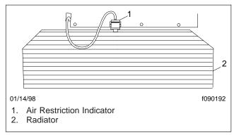
Fig. 2, Air Restriction Indicator Location
