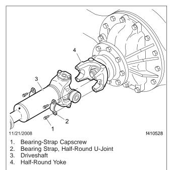
Fig. 1, Half-Round U-Joint Installation
