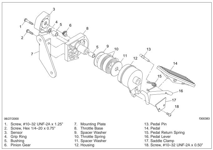
Fig. 2, Electronic Throttle Pedal Assembly (exploded view)
