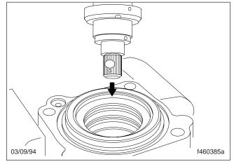
Fig. 59, Lubricate, then Install the Input-Shaft/Valve/ Worm Assembly
