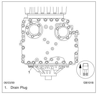
Fig. 2, Transmission Drain Plug (bottom view)
