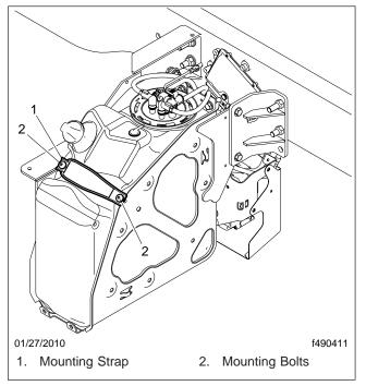
Fig. 2, 13-Gallon Tank Mounting
