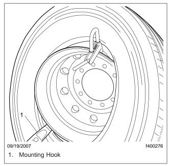
Fig. 6, Mounting Hook Placement
