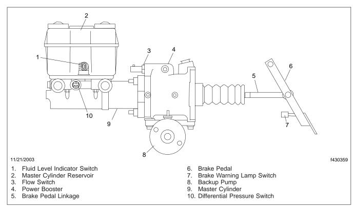
Fig. 4, Components of the Master Cylinder and Power Brake Booster
