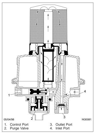
Fig. 1, Drying Cycle
