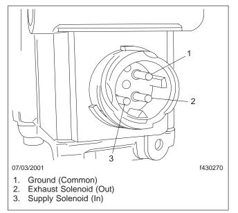
Fig. 3, Modulator Valve Terminals
