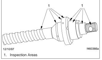
Fig. 42, Inspect the Upper Shaft-Seal Area
