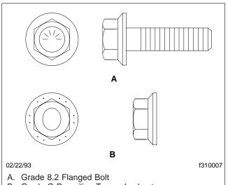
B. Grade G Prevailing Torque Locknut
