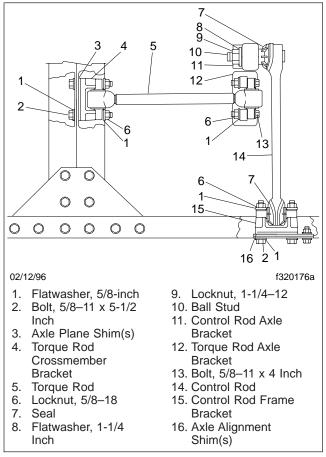
Fig. 1, Torque Rod Mounting
