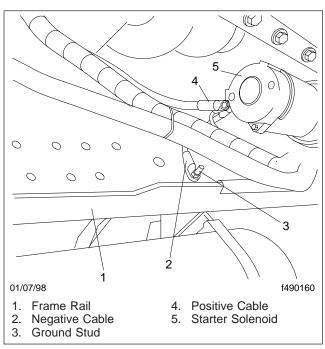
Fig. 1, Battery Cables
