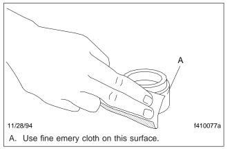
Fig. 16, Smoothing a Half-Round Yoke U-Joint Bearing Cup
