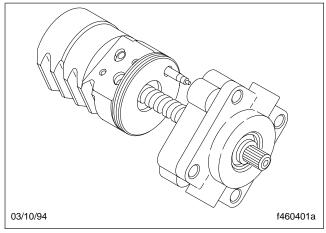
Fig. 75, Insert the Worm Shaft and Input Shaft Assembly
