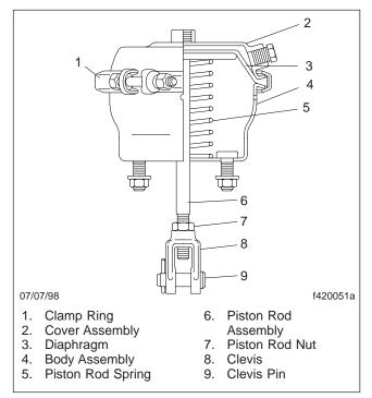
Fig. 1, Brake Chamber (sectional view)
