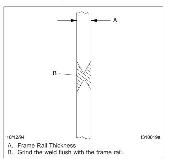
Fig. 8, Second Weld Ground Flush
