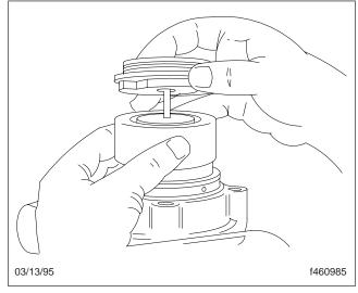
Fig. 9, Removing the Top Plate
