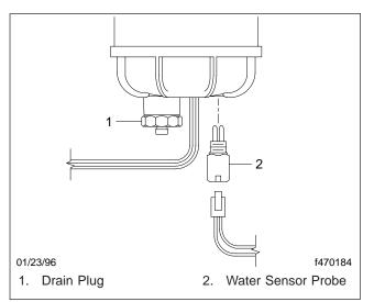
Fig. 1, Water Sensor Probe
