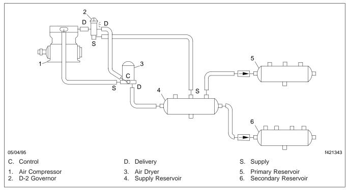
Fig. 2, Standard Air Dryer Plumbing Diagram
