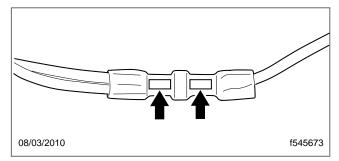
Fig. 2, Properly Crimped Splice
