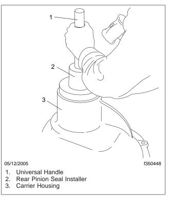
Fig. 3, Installing the Rear Pinion Seal
