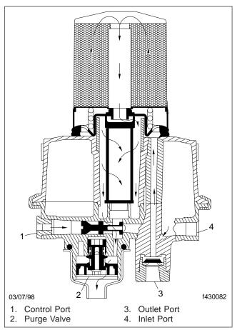
Fig. 2, Purging Cycle
