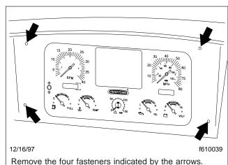
NOTE: A typical instrument cluster installation is shown; the procedure is the same for all installations.
