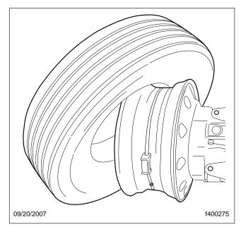
Fig. 5, Passing Both Beads Over the Rim Flange at the Same Time
