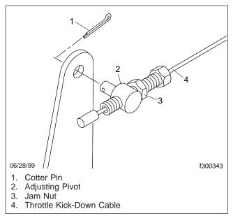
Fig. 1, Throttle Kick-Down Cable Adjusting Pivot
