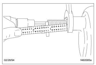
Fig. 7, Back Out the Adjusting Screw and Measure
