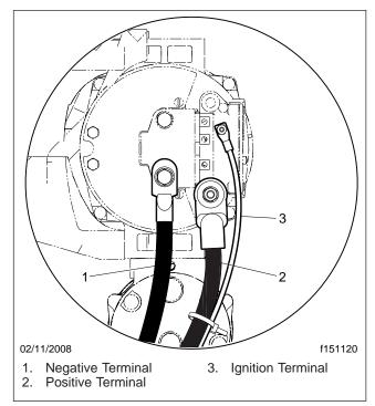
Fig. 2, 4940 Pad-Mount Alternator Terminals
