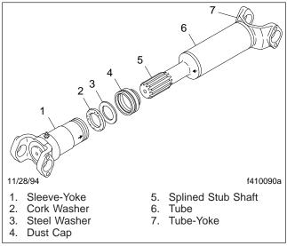
Fig. 6, Slip-Joint Components
