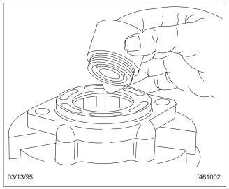
Fig. 27, Installing the Seal in the Cover
