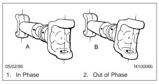
Fig. 4, U-Joint Phasing
