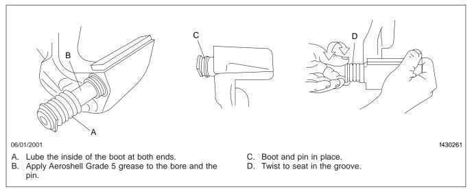
Fig. 6, Installing Guide Pins and Boots
