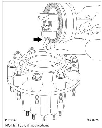
Fig. 5, Seat the Seal in the Tool
