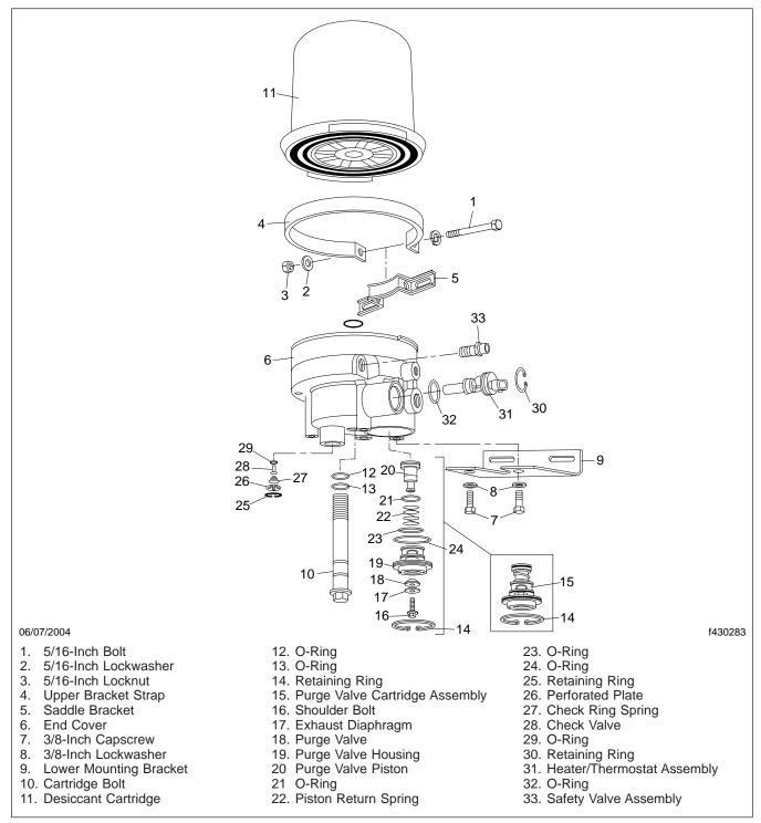
Fig. 1, AD-IP (exploded view)
