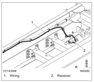
Fig. 2, TPMS Wiring to the Receiver
