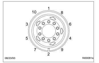
Fig. 4, 10-Stud Disc Wheel Tightening Sequence
