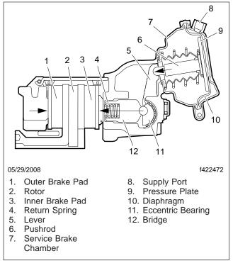
Fig. 1, Bendix Air Disc Brake
