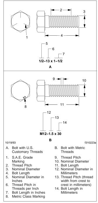
Fig. 1, Fastener Size and Thread Identification
