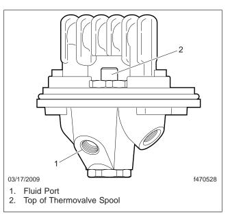
Fig. 4, Fluid Heater Thermovalve Test
