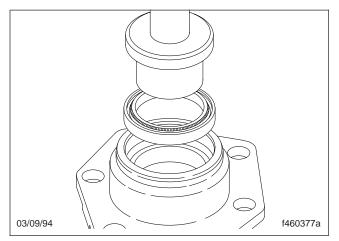
Fig. 52, Put the New Seal on Special Tool
