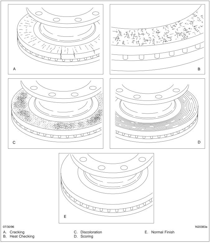
Fig. 5, Rotor Surface Check
