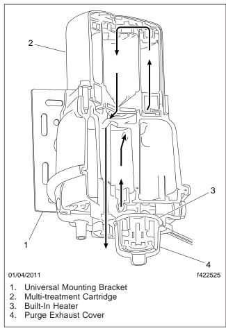
Fig. 2, PURest Charge Cycle
