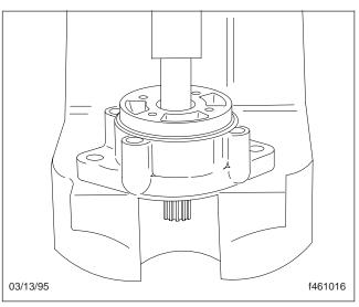
Fig. 20, Pressing the Needle Bearing out of the Cover
