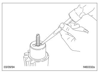
Fig. 12, Unstake the Adjusting-Screw Retainer
