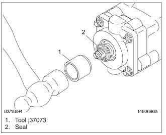
Fig. 100, Tap the Seal Into the Valve Housing Bore
