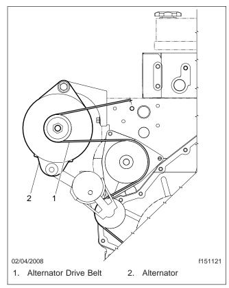
Fig. 1, Cummins ISB Alternator Mounting
