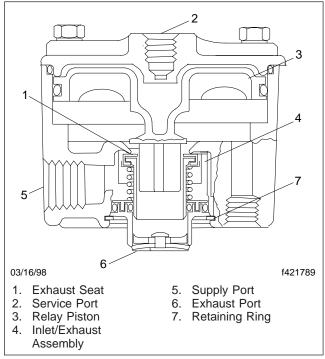
Fig. 3, R-12 Relay Valve (sectional view)
