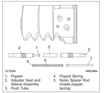
Fig. 24, Remove the Poppets, Spring, Spacer Rod, and Push Tube
