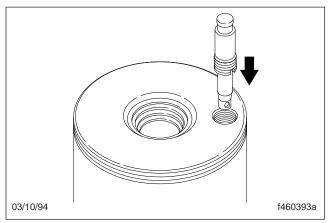
Fig. 67, Screw the Poppet Adjuster Seat and Sleeve Assembly into the Rack Piston
