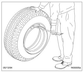
Fig. 3, Prying the Rim Out of the Tire
