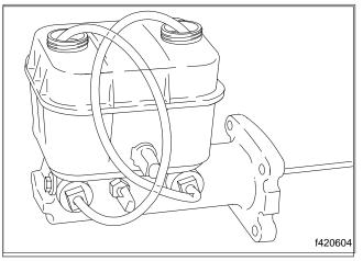
Fig. 5, Outlet Ports With Master Cylinder Bleeder Tubes
