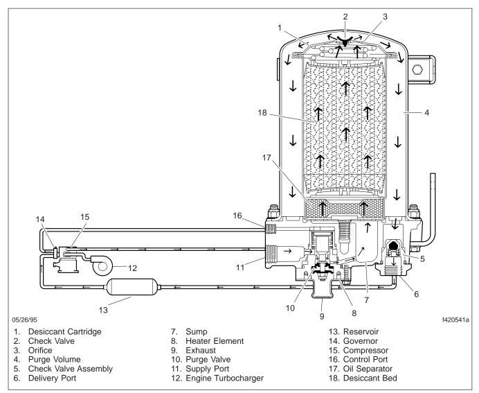
Fig. 3, AD-9 Charge Cycle
