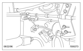
Fig. 1, Injection Pump Lever and Yokes
