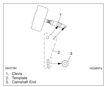
Fig. 8, Position the Installation Template
