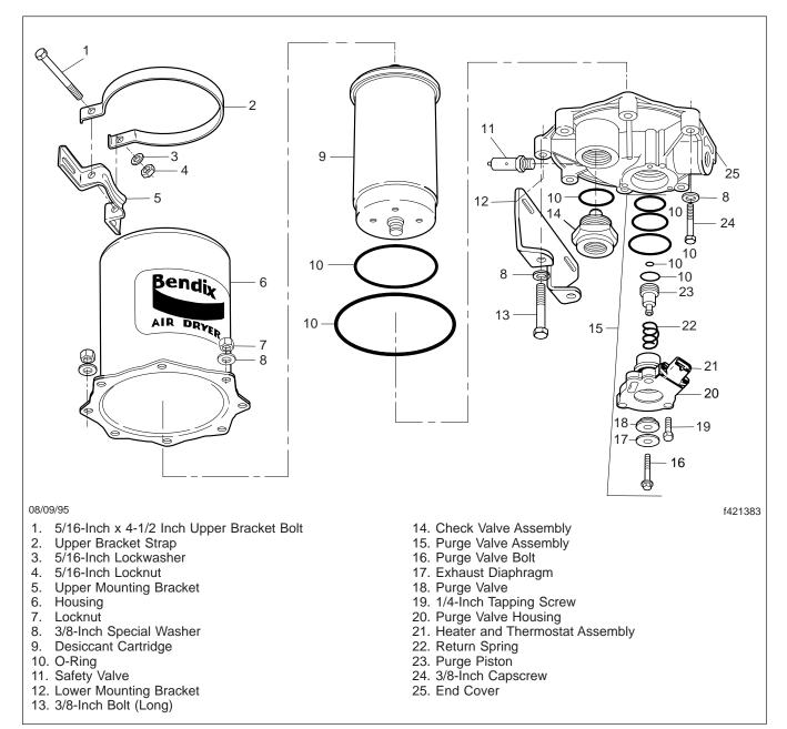
Fig. 1, AD-9 (exploded view)
