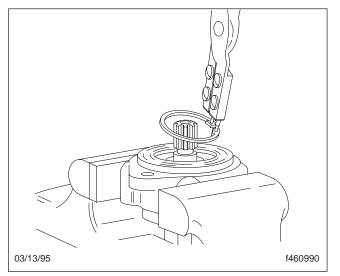
Fig. 14, Removing the Large Retaining Ring
