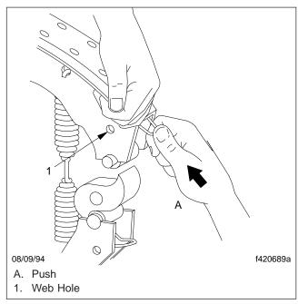
Fig. 7, Push the Retainer into the Brake Shoe
