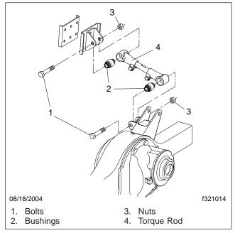
Fig. 3, Torque Rod Removal/Installation
