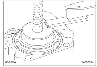
Fig. 62, Install the Bearing Adjuster over the Worm Shaft
