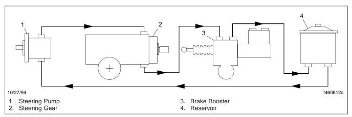
Fig. 1, Steering System With Hydraulic Brakes
