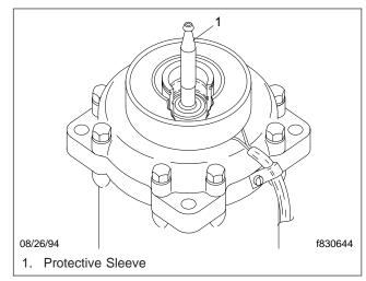
Fig. 3, Position the Shaft Seal Protective Sleeve
