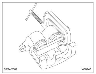
Fig. 6, Retracting Pistons Into the Caliper
