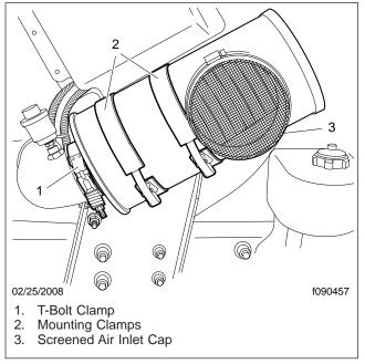
Fig. 1, Farr ECO SE Air Cleaner (front-mounted)
