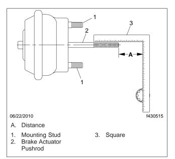
Fig. 4, Measuring the Brake Actuator Pushrod
