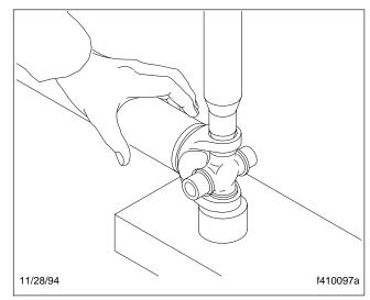
Fig. 3, Pressing the U-Joint Out-of/Into a Yoke
