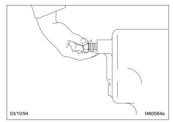
Fig. 80, Install a new Poppet Stopscrew
