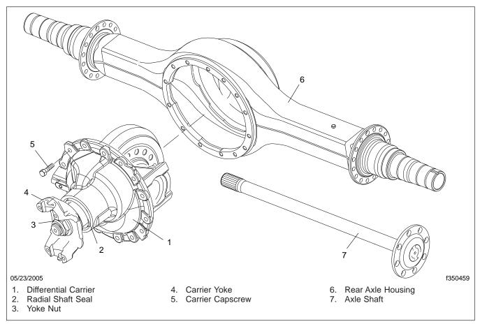
Fig. 1, Single Axle Components
