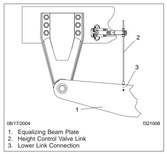
Fig. 1, Height Control Valve Linkage
