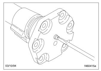
Fig. 89, Install the Sector Shaft Adjusting Screw
