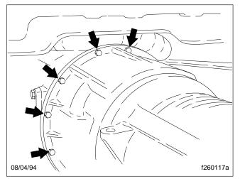
Fig. 7, Transmission Flange Bolts
