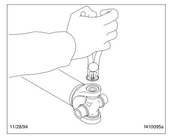
Fig. 2, Removing/Installing the U-Joint Snap Ring
