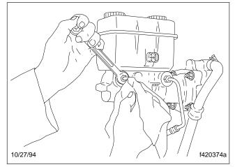
Fig. 4, Loosening the Fitting at the Front Outlet Port
