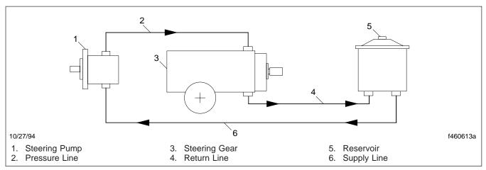
Fig. 2, Steering System With Air Brakes
