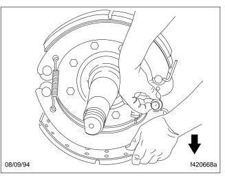
Fig. 1, Remove the Bottom Cam Roller
