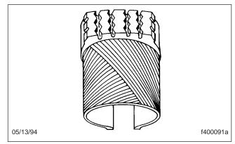
Fig. 3, Bias Ply Tire Construction
