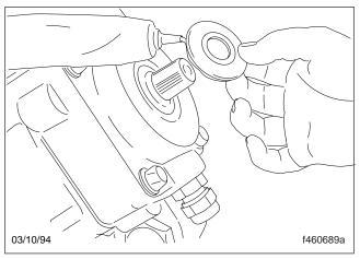
Fig. 102, Install the Dirt-and-Water Seal
