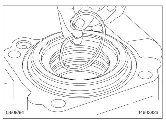
Fig. 57, Lubricate and Install a New Large Diameter O-Ring and a New Seal Ring
