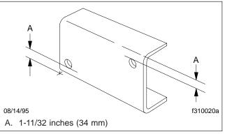
Fig. 9, Minimum Distance for Drilling Holes
