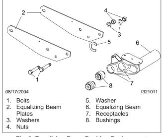
Fig. 3, Equalizing Beam Bushing Replacement
