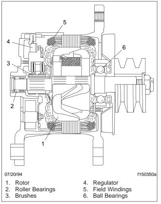
Fig. 2, Delco Remy 21-SI Alternator (cutaway view)
