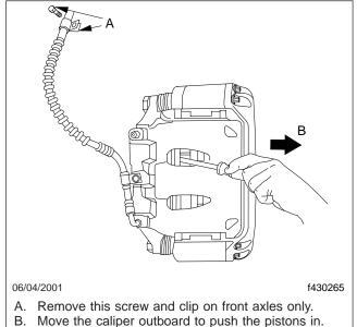
B. Move the caliper outboard to push the pistons in.
