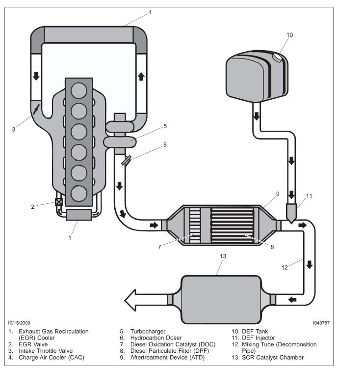
Fig. 1, EPA10 Aftertreatment System (typical)
