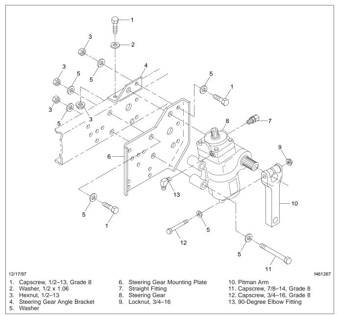
Fig. 1, Power Steering Gear Installation
