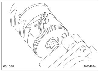
Fig. 76, Install New Ball Return Guide Halves
