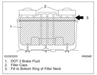
Fig. 6, Master Cylinder Fill Level
