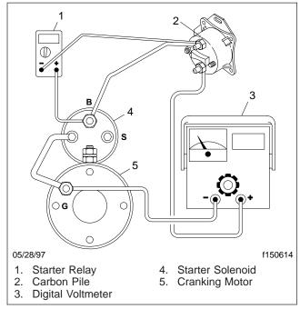
Fig. 5, Starter Wiring Test-Second Wire Voltage Loss (V6)
