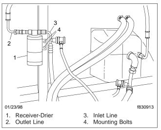
Fig. 1, Receiver-Drier
