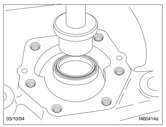
Fig. 88, Press in the New Seal
