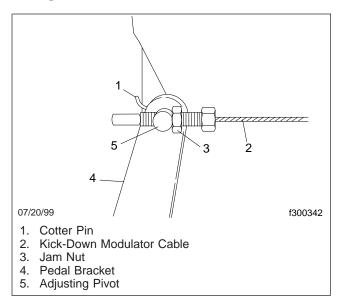
Fig. 1, Kick-Down Modulator Cable Pedal Connection (with non-electronic automatic transmission)
