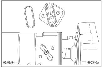
Fig. 17, Remove the Cap and Seal
