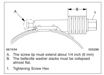
Fig. 2, Breeze Constant-Torque Hose Clamp
