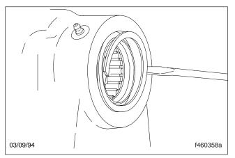
Fig. 34, Remove the Retaining Ring
