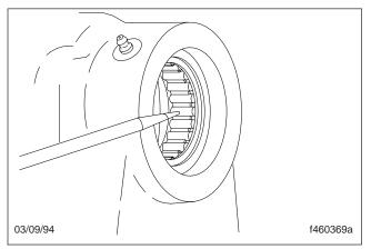
Fig. 45, Inspect the Housing Roller Bearing
