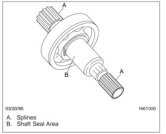
Fig. 23, Checking the Input Shaft
