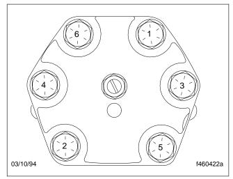
Fig. 96, Six-Bolt Tightening Sequence
