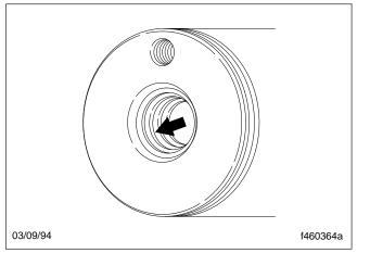
Fig. 40, Inspect the Rack Piston Internal Ball-Track Grooves
