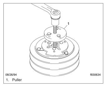
Fig. 3, Remove the Drive Plate
