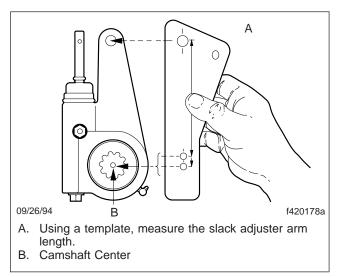
Fig. 5, Slack Adjuster Measurement
