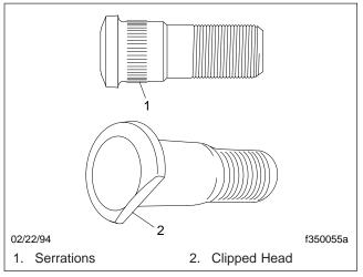
Fig. 5, Typical Headed Wheel Studs
