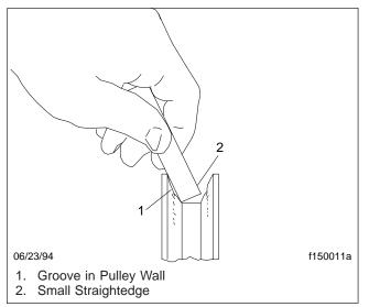
Fig. 2, Check for Pulley Wear
