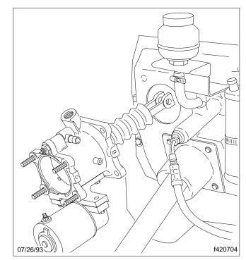
Fig. 5, Power Brake Booster Removal
