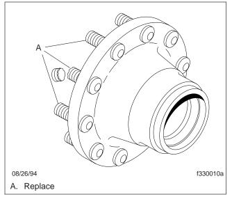
Fig. 1, Studs to Replace
