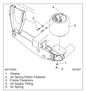
Fig. 2, Air Spring Assembly
