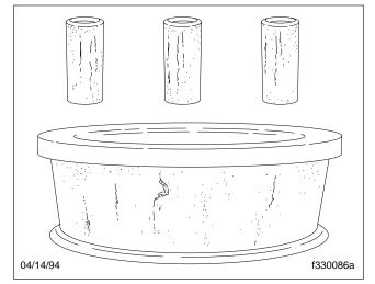
Fig. 12, Etching (Pitting) on Bearing Surfaces
