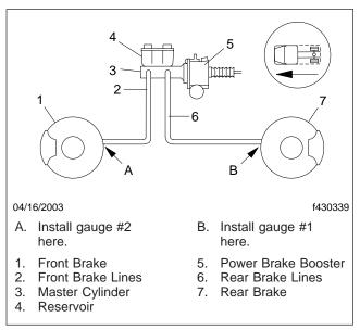
Fig. 1, Gauge Installation
