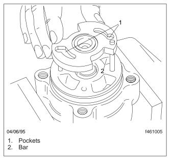
Fig. 30, Installing the Bottom Plate
