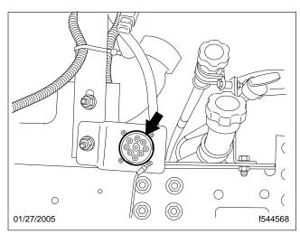
Fig. 1, Rear Diagnostic Connector (actual location will vary)
