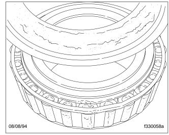
Fig. 11, Bearing Damage Resulting from Inadequate Lubrication
