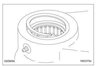
Fig. 54, Install the Second Retaining Ring
