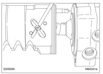
Fig. 18, Remove the Ball Return Guide Halves
