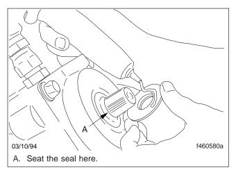
Fig. 8, Install the Dirt-and-Water Seal
