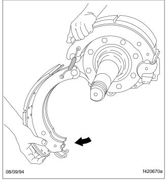
Fig. 3, Remove the Springs and Brake Shoes
