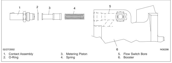
Fig. 1, Flow Switch Assembly (exploded view)
