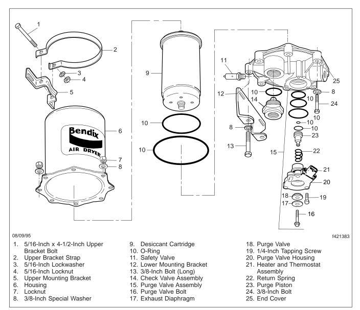
Fig. 1, Bendix AD-9 Air Dryer
