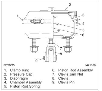
Fig. 1, Brake Chamber (sectional view)
