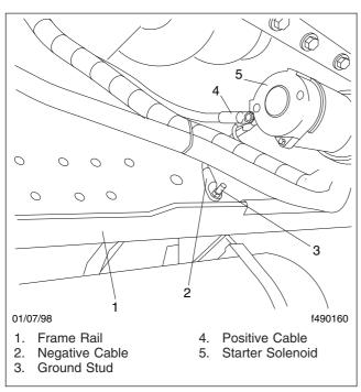
Fig. 1, Battery Cables
