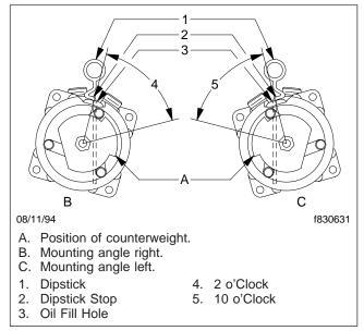
Fig. 1, Checking the Oil Level
