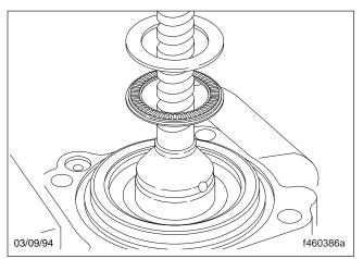
Fig. 60, Lubricate, then Install a Second Thrust Bearing and Thin Washer
