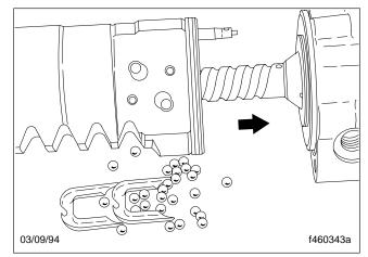
Fig. 20, Remove the Worm Shaft and Valve Housing Assembly
