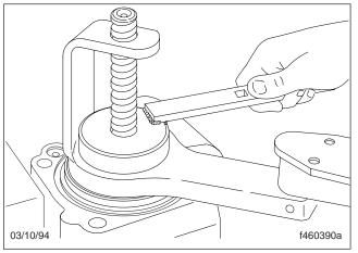
Fig. 64, Install the Locknut on the Bearing Adjuster
