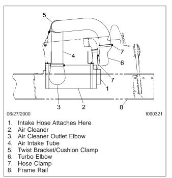
Fig. 2, Air Intake Ducting (side view)
