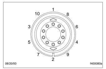
Fig. 1, 10-Stud Disc Wheel Tightening Sequence
