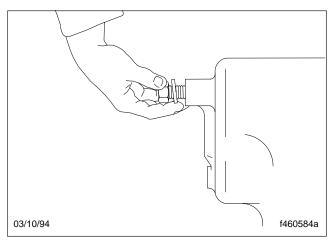
Fig. 4, Remove the Poppet Fixed Stopscrew and Washer
