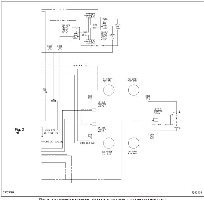
Fig. 3, Air Plumbing Diagram, Chassis Built From July 1997 (partial view)
