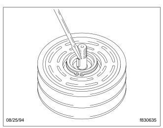
Fig. 4, Remove the Shaft Key
