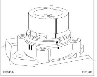
Fig. 31, Installing the Cam Ring
