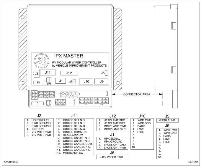
Fig. 2, Multiplex IPX Master Controller
