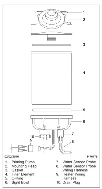
Fig. 1, Fuel/Water Separator Assembly
