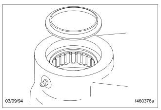
Fig. 53, Install the New Dirt Seal
