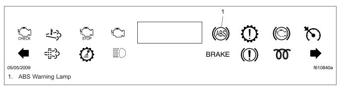
Fig. 4, ABS Lamp (Lightbar Control Unit [LBCU] instrument panel shown)
