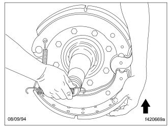
Fig. 2, Remove the Spring
