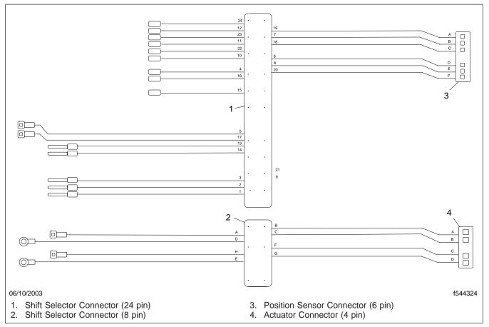
Fig. 1, Shift-by-Wire (SBW) Wiring Diagram
