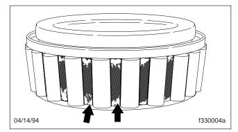
Fig. 8, Rubbing Marks on Bearing Cage
