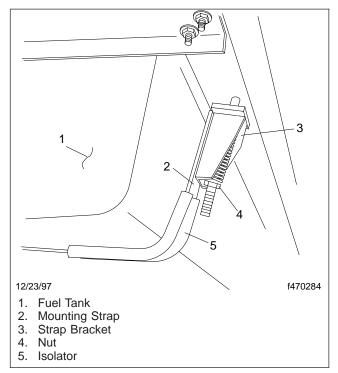
Fig. 1, Fuel Tank Mounting Strap Assembly
