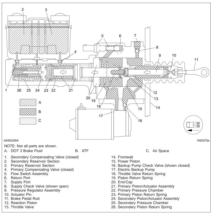
Fig. 7, Power Brake Booster and Master Cylinder
