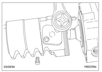
Fig. 16, Remove the Two Sealing Screws
