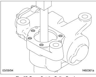
Fig. 37, Press Out the Roller Bearings
