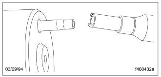
Fig. 22, Slide the Special Tool Over the Poppet Adjuster Seat
