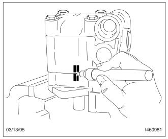
Fig. 5, Marking the Housing and the Cover
