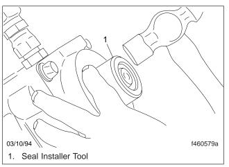
Fig. 7, Position the Seal Installer Tool
