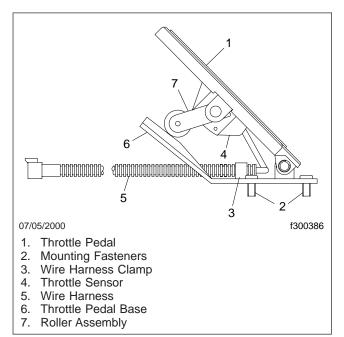
Fig. 1, Felsted Electronic Throttle Pedal (left-side view)
