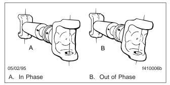
Fig. 3, U-Joint Phasing
