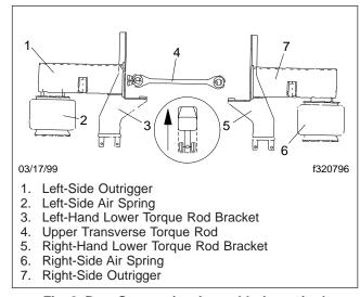
Fig. 3, Rear Suspension Assembly (rear view)
