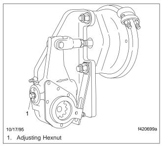
Fig. 5, Turn the Adjusting Hexnut Clockwise
