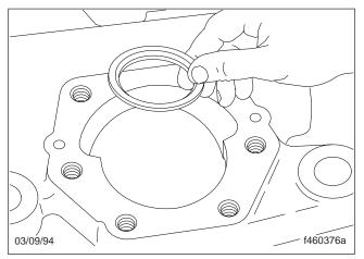
Fig. 51, Put the Gear Housing on its Side (with the side-cover end of the bore facing up)
