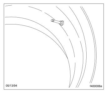
Fig. 4, Valve Stem Installation
