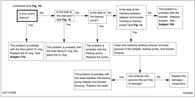
Fig. 11, Flow Chart: Hydraulic System Leakage (cont.)
