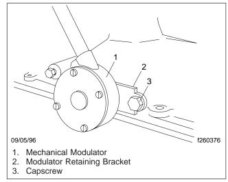
Fig. 3, Mechanical Modulator
