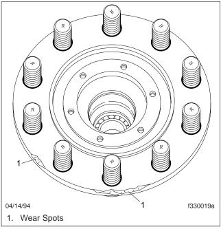
Fig. 1, Damaged Front Axle Wheel Hub
