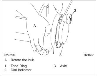
Fig. 4, Checking Tone-Ring Runout
