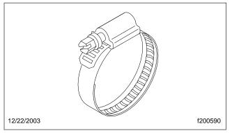
Fig. 3, ABA Radial-Worm-Drive Hose Clamp (typical)
