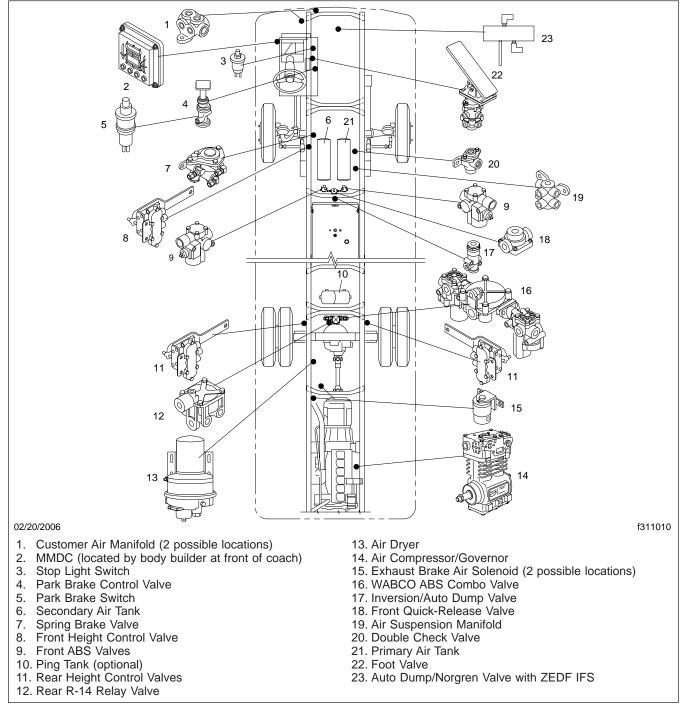
Fig. 1, Air Plumbing Component Locations, MMDC Chassis
