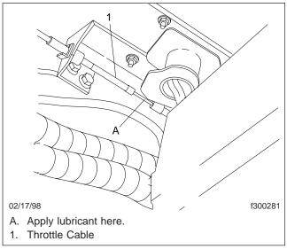
Fig. 1, Throttle Cable Lubrication
