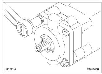
Fig. 14, Remove the Valve Housing Bolts
