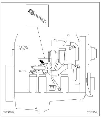
Fig. 1, Block Heater Element Installation (typical)
