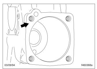
Fig. 44, Inspect the Housing Faces for Nicks
