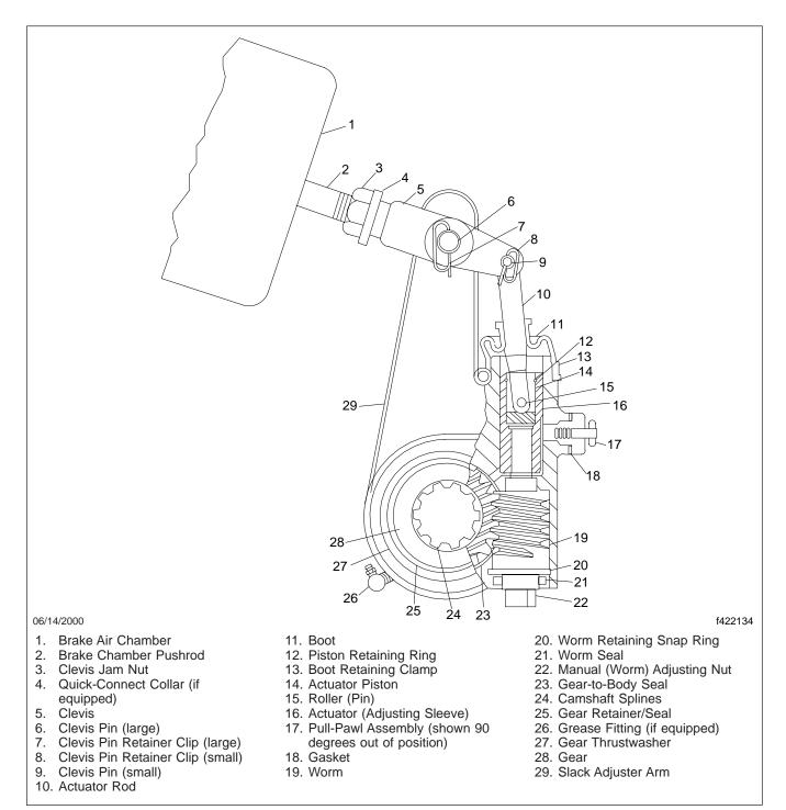
Fig. 1, Automatic Slack Adjuster (sectional view)
