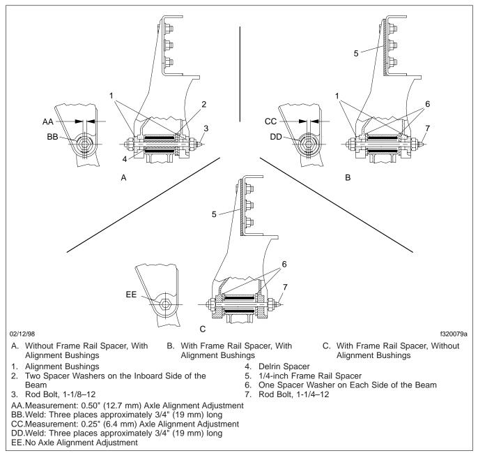
Fig. 2, Spacer Washer Installation and Alignment Bushing Welding
