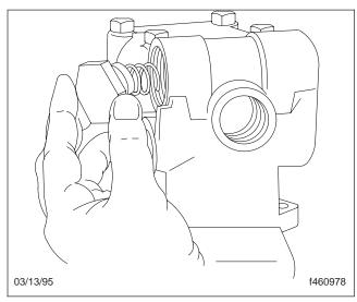
Fig. 2, Removing the End Plug
