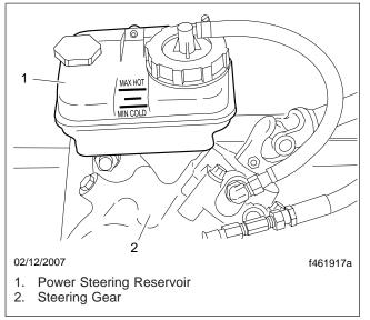
Fig. 6, Fluid Level Check
