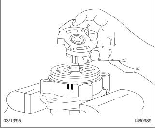
Fig. 13, Removing the Bottom Plate
