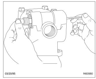
Fig. 4, Removing the Control Valve Assembly
