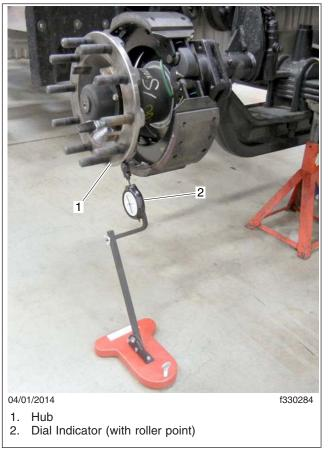
Fig. 2, Setup to Measure Radial Runout
