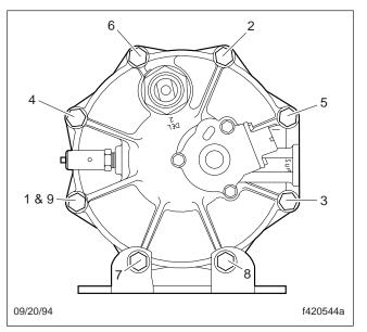
Fig. 2, End Cover to Housing Torque Pattern
