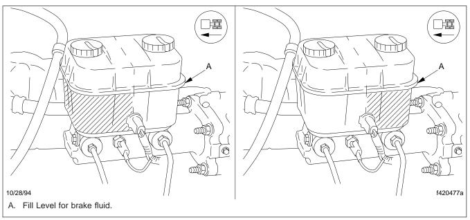
Fig. 1, Master Cylinder Reservoir
