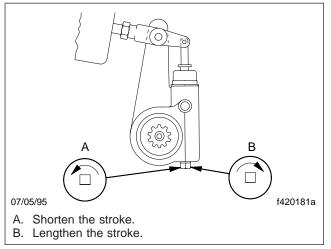
Fig. 4, Turn the Adjusting Nut
