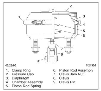
Fig. 1, Brake Chamber (sectional view)
