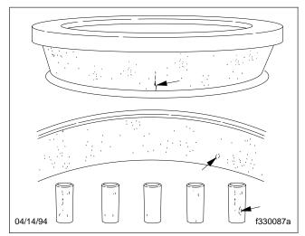
Fig. 10, Indentations, Cracks, or Breaks in Bearing Surfaces
