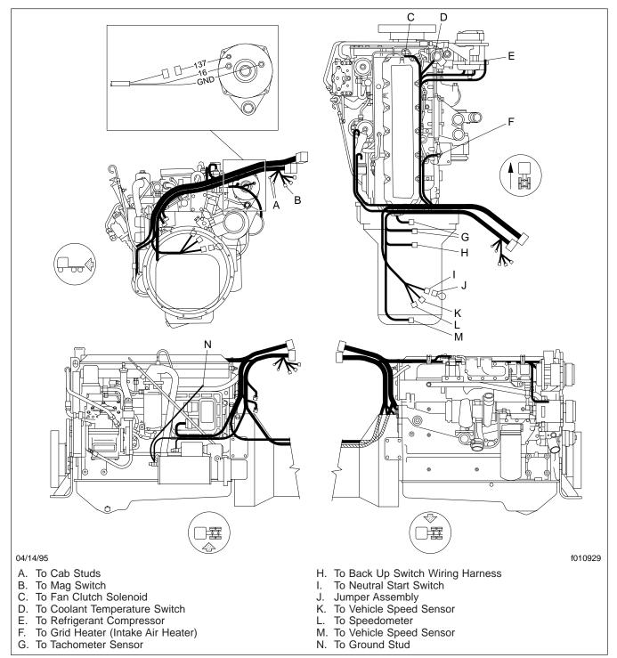
Fig. 1, Wiring Harnesses
