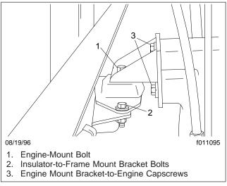
Fig. 3, Rear Engine Mount
