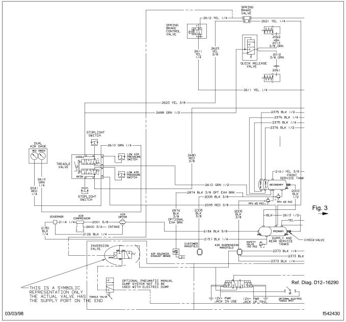
Fig. 2, Air Plumbing Diagram, Chassis Built From July 1997 (partial view)
