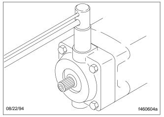
Fig. 85, Turn the Relief Valve Cap into the Valve Housing
