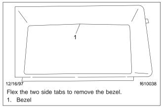
Fig. 1, Instrument Panel Bezel
