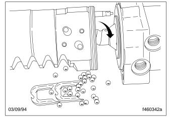
Fig. 19, Remove the Steel Balls
