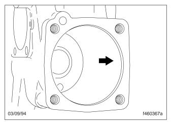
Fig. 43, Inspect the Housing Cylinder Bore
