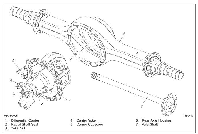
Fig. 1, Single Axle Components
