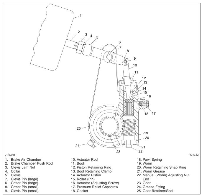
Fig. 1, Automatic Slack Adjuster (sectional view)
