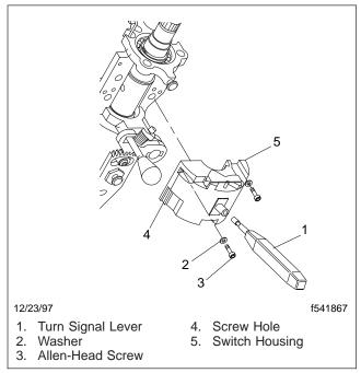
Fig. 1, Turn Signal Switch
