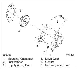
Fig. 1, Vickers Pump Mounting
