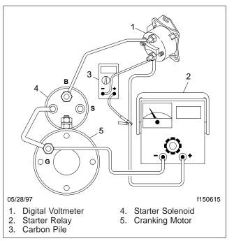
Fig. 4, Starter Wiring Test-First Wire Voltage Loss (V5)
