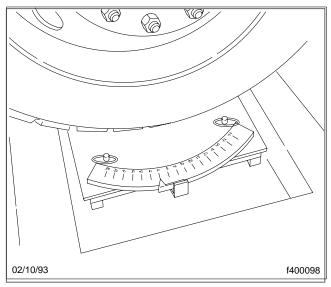
Fig. 2, Turn-Plate (Turntable), Stationary Type
