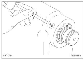
Fig. 103, Install a New Grease Fitting
