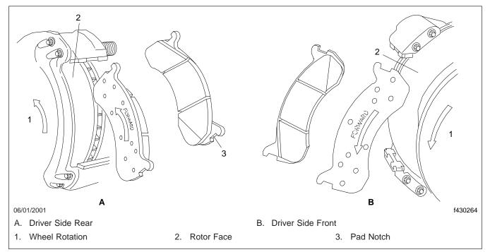
Fig. 7, Replacing Brake Pads on Front and Rear Brakes
