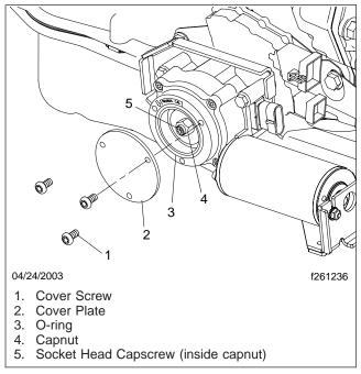
Fig. 1, Cover Plate and Capnut
