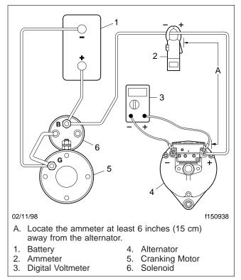
Fig. 3, Setup 2: Alternator Output Test
