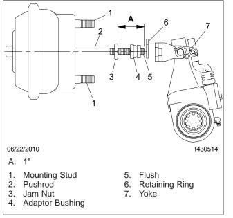
Fig. 3, Quick-Connect Yoke Assembly
