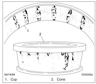
Fig. 3, Spalling (Flaking) of Wheel Bearing Assembly
