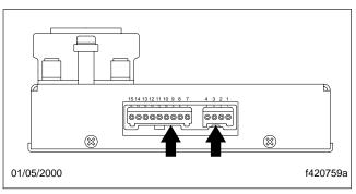
Fig. 6, Monitor Module Terminals
