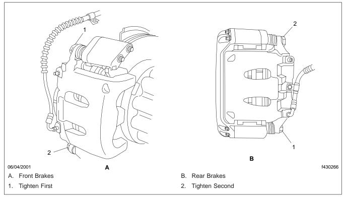
Fig. 9, Tightening Sequence for Caliper Mounting Bolts
