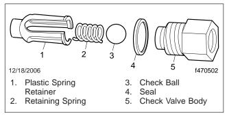
Fig. 3, Check Valve Assembly
