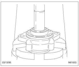
Fig. 28, Pressing the Shaft and Bearing into the Cover
