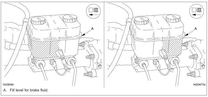
Fig. 1, Master Cylinder Reservoir
