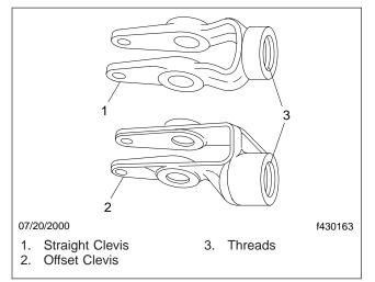
Fig. 2, One-Piece Threaded Clevis Configurations
