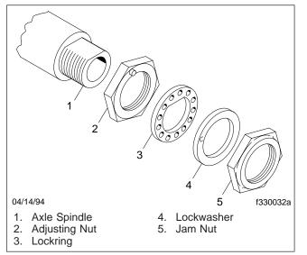
Fig. 2, Axle With Jam Nut and Lockring
