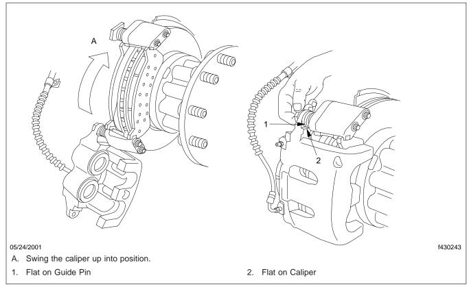
Fig. 8, Closing the Caliper Over Brake Pads and Rotor
