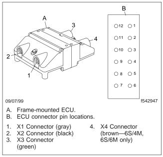
Fig. 3, ECU Module, and Pin Locations in the Connector
