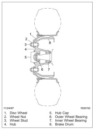
Fig. 1, Hub and Wheel Assembly
