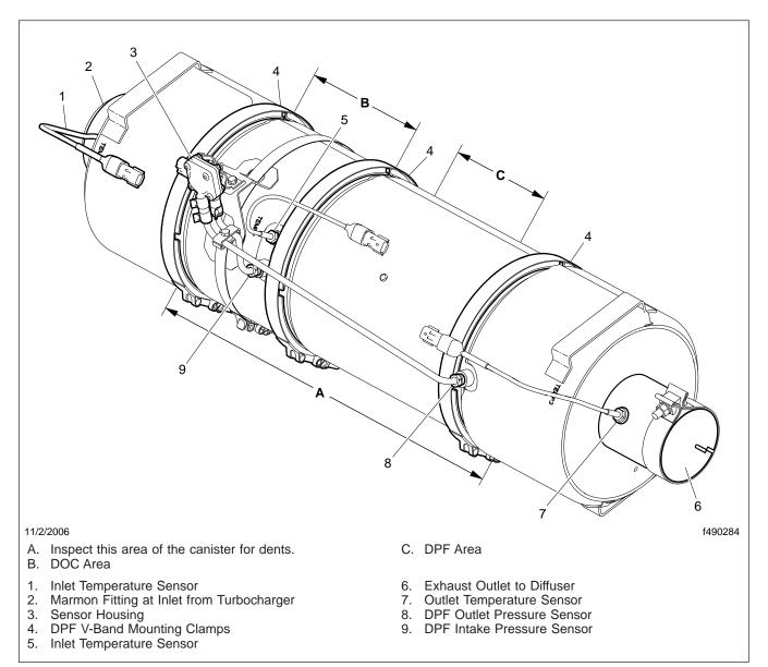
Fig. 1, Aftertreatment Device (typical)
