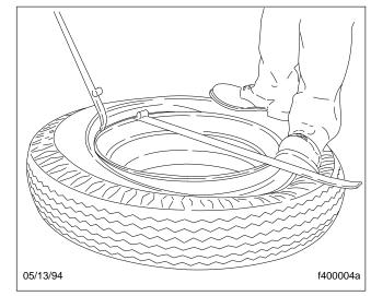
Fig. 2, Forcing Bead into the Rim Well
