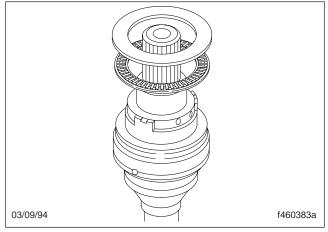
Fig. 58, Install the Roller Thrust Bearing and the Thick Thrustwasher
