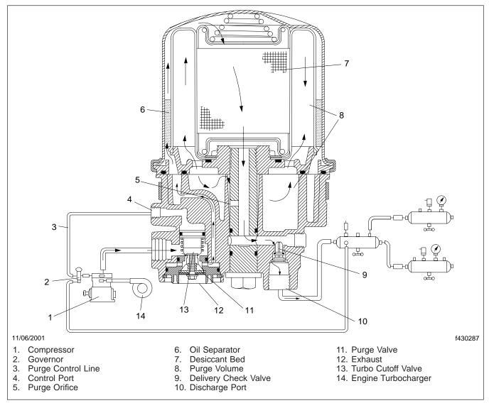
Fig. 2, AD-IP Charge Cycle
