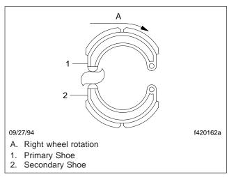
Fig. 1, Camshaft Behind Axle
