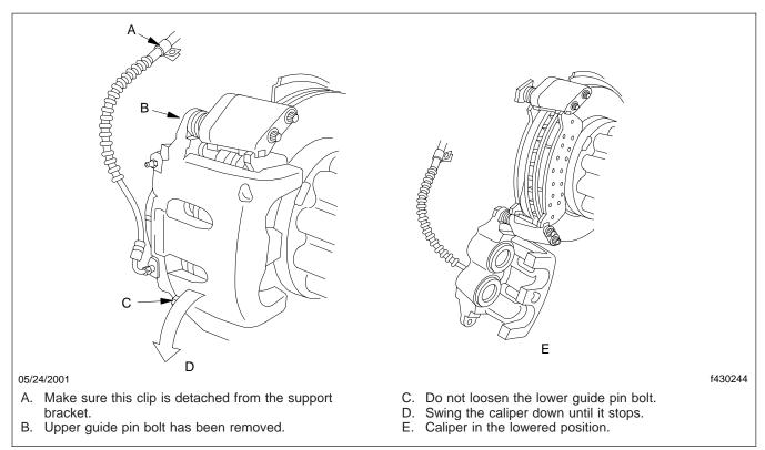
Fig. 4, Opening the Caliper to Access Brake Pads and Pistons
