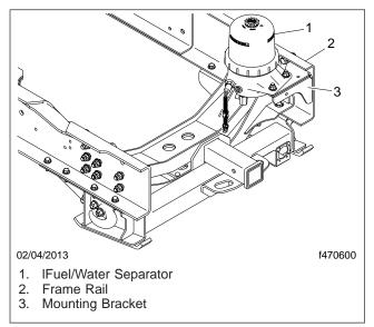
Fig. 1, Davco Fuel/Water Separator Location
