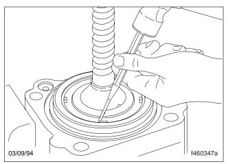
Fig. 25, Unstake the Adjuster Locknut
