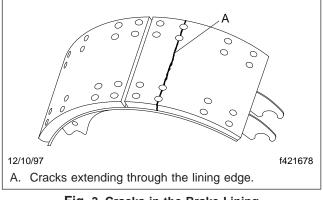
Fig. 3, Cracks in the Brake Lining
