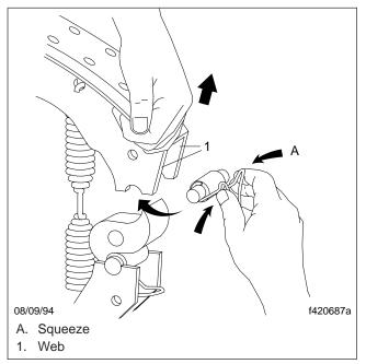
Fig. 6, Install the Cam Rollers and Retainers
