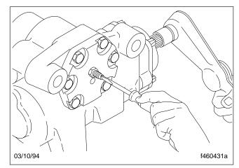
Fig. 105, Adjust the Sector Shaft Adjusting Screw
