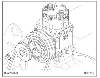
Fig. 4, Two-Cylinder Reciprocating Compressor
