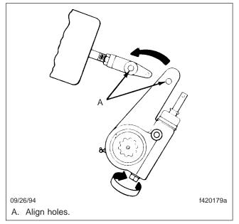
Fig. 7, Aligning the Holes
