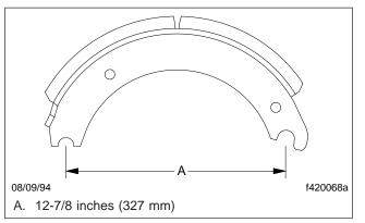
Fig. 7, Measuring the Shoe Span
