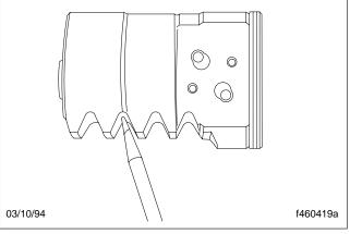
Fig. 93, Check the Tooth Space
