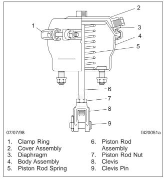
Fig. 1, Brake Chamber (sectional view)
