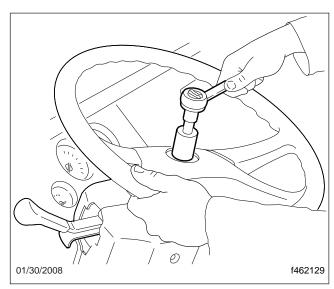
Fig. 2, Removing the Steering Wheel Nut
