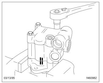
Fig. 6, Removing the Screws and Washers
