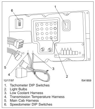
Fig. 1, Back of Instrument Cluster
