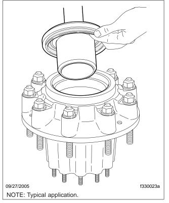
Fig. 6, Insert the Tool
