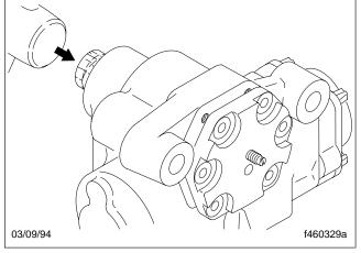
Fig. 9, Remove the Side Cover and Sector Shaft
