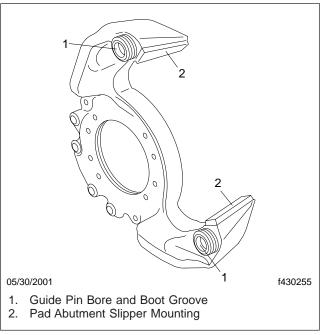
Fig. 4, Anchor Plate Machined Surfaces
