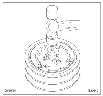
Fig. 9, Install the Drive Plate Assembly
