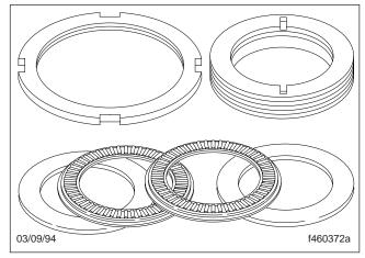
Fig. 48, Inspect the Thrust Bearing Rollers and Thrustwashers
