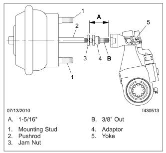
Fig. 3, Easy-On Yoke Assembly
