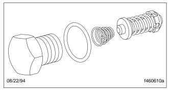
Fig. 84, Install the Tapered Spring
