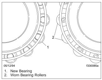
Fig. 6, Wheel Bearing Roller Wear
