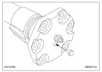
Fig. 91, Press in a New Rubber Plug
