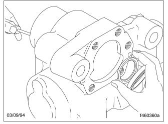
Fig. 36, Push the Seal and the Spacer Washer
