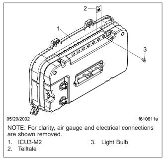
Fig. 3, ICU3-M2, Rear View (exploded)
