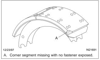
Fig. 5, Portions of the Brake Lining Missing
