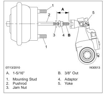
Fig. 2, Easy-On Yoke Assembly
