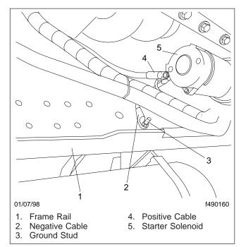
Fig. 2, Battery Cables
