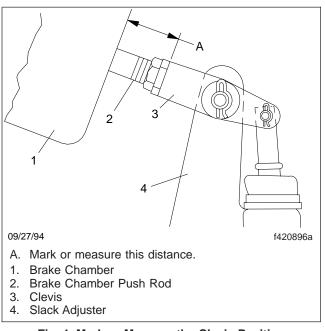
Fig. 1, Mark or Measure the Clevis Position
