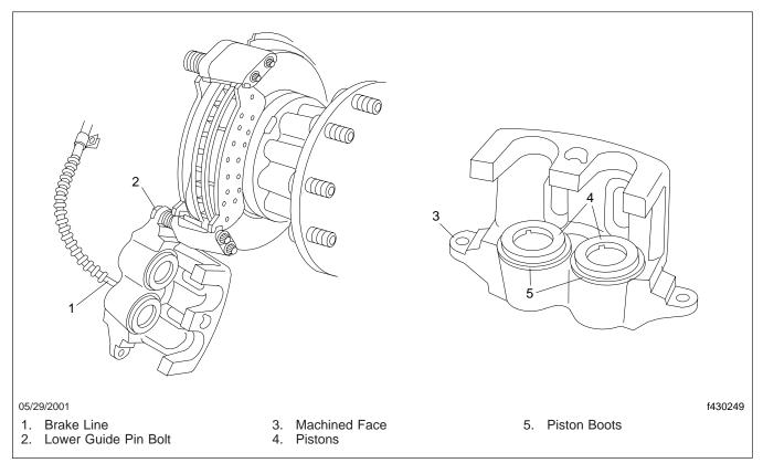
Fig. 4, Removing the Caliper from the Anchor Plate
