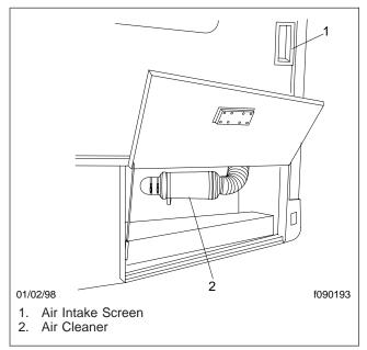
Fig. 1, Air Cleaner and Air Intake Screen
