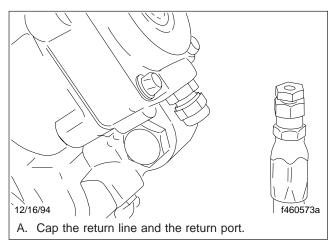
Fig. 1, Disconnect the Return Line
