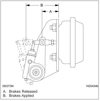
Fig. 1, Measure the Distance Between A and B
