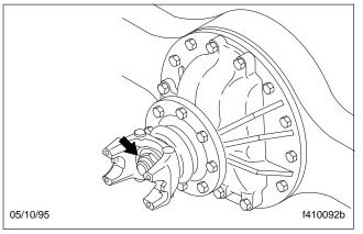
Fig. 7, Axle End-Yoke Locknut
