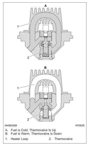
Fig. 3, Heat Exchanger Fluid Flow
