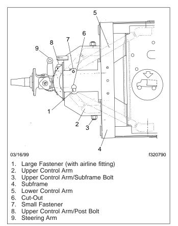
Fig. 4, Front Suspension Assembly (overhead view)
