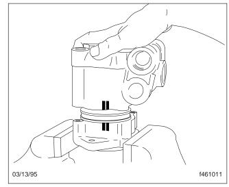
Fig. 36, Installing the Housing
