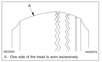
Fig. 2, Tire Damage Due to Excessive Camber
