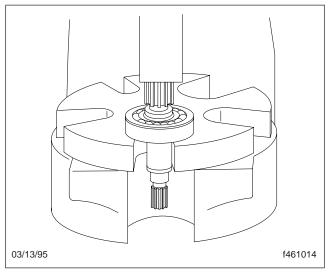
Fig. 25, Pressing the Input Shaft
