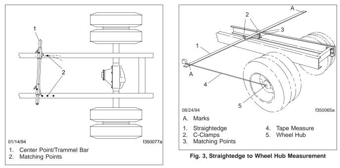
Fig. 2, Marking an Arc
