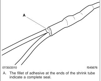
Fig. 5, Completed Three-Wire Tap Splice
