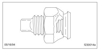
Fig. 1, Damaged Outer Wheel Nut
