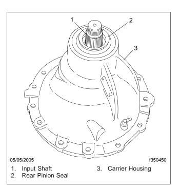
Fig. 2, Rear Pinion Seal
