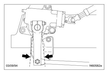
Fig. 2, Checking Sector Shaft Free-Play
