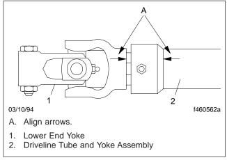
Fig. 2, Driveline Alignment
