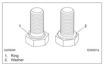
Fig. 8, Integral Ring and Washer
