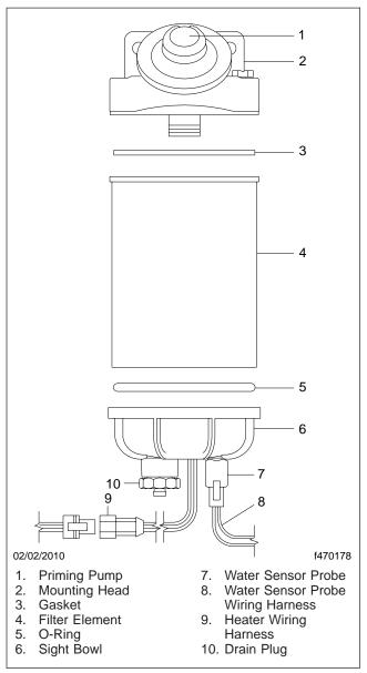
Fig. 4, Fuel/Water Separator Assembly
