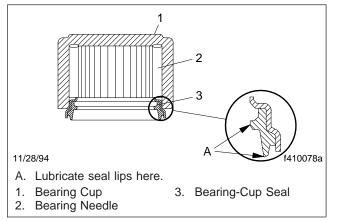
Fig. 15, Sectional View of a Half-Round End-Yoke U-Joint Bearing Cup
