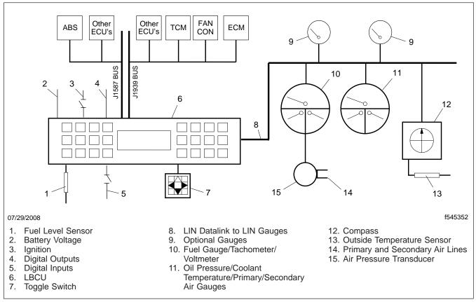
Fig. 1, Problems Diagnosed Through the LBCU
