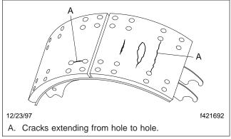
Fig. 6, Cracks in the Brake Lining
