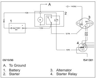
Fig. 1, Charging Circuit Wiring
