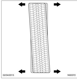
Fig. 1, Lateral Runout
