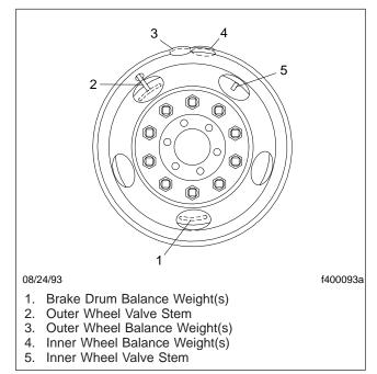
Fig. 3, Alternate Location of Wheel and Brake Drum Balance Weights, Five-Handhole or Aluminum Wheels
