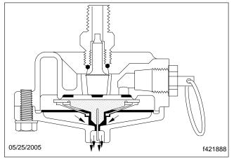
Fig. 5, Exhaust Cycle
