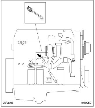
Fig. 1, Block Heater Element Installation (typical)
