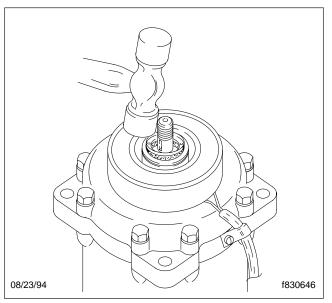
Fig. 5, Tap the New Felt Ring in Place
