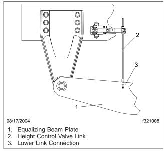
Fig. 1, Height Control Valve Linkage
