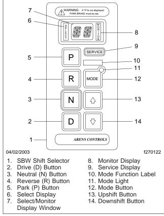
Fig. 1, SBW Push-Button Shift Selector (1000/2400 series)
