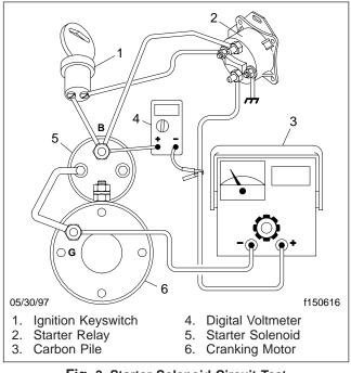
Fig. 3, Starter Solenoid Circuit Test
