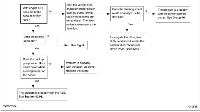
Fig. 8, Flow Chart: Brake Pedal Feels Very Hard
