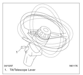
Fig. 2, Tilt/Telescoping Steering Column
