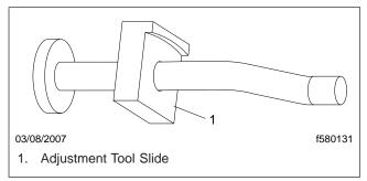
Fig. 1, ABS Sensor Adjustment Tool
