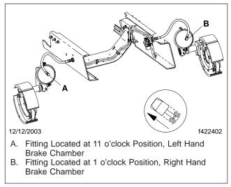
Fig. 2, Brake Chamber Fitting Position
