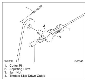
Fig. 1, Throttle Kick-Down Cable Adjusting Pivot
