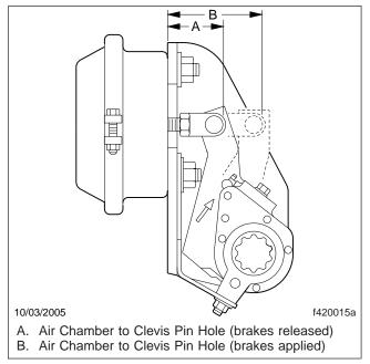
Fig. 6, Brake Stroke Check, Haldex (SAB) Automatic Slack Adjuster
