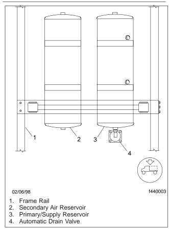
Fig. 1, Front Air Reservoirs (typical location)
