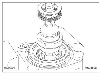
Fig. 28, Remove the Thin Washer, Thrust Bearing, Input Shaft, Rotary Valve, and Worm Shaft Assembly
