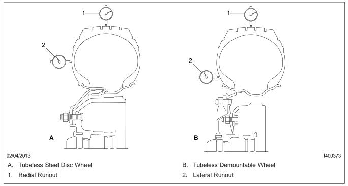
Fig. 3, Runout Check for Tires
