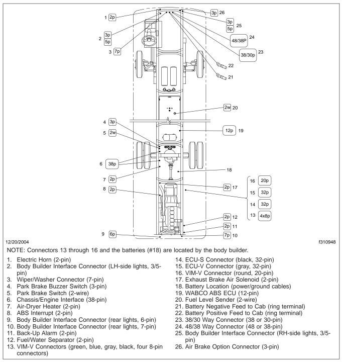
Fig. 2, Electrical Connector and Component Locations
