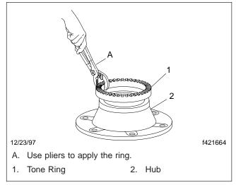
Fig. 1, Installing the Ring on the Hub
