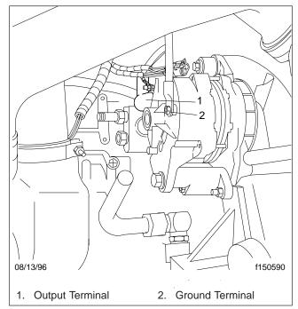
Fig. 4, Electrical Connectors
