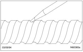
Fig. 41, Inspect the Worm Shaft Ball-Track Grooves
