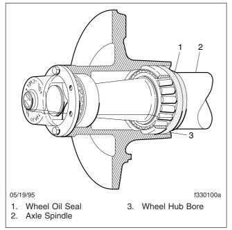
Fig. 1, Wheel Oil Seal
