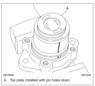
Fig. 33, Installing the Top Plate
