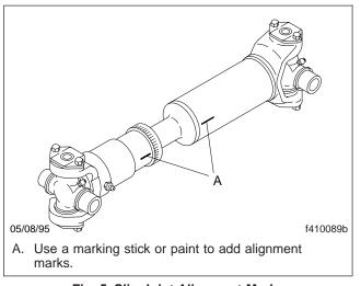
Fig. 5, Slip-Joint Alignment Marks
