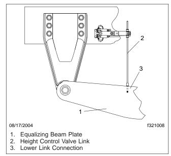
Fig. 2, Height Control Valve Linkage
