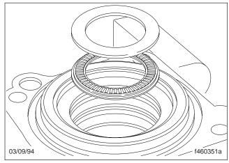
Fig. 29, Remove the Roller Thrust Bearing and Thick Thrustwasher
