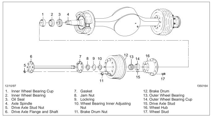
Fig. 4, Typical Drive Axle (exploded view)
