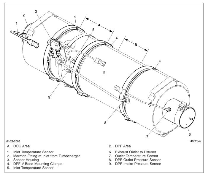
Fig. 1, Aftertreatment Components (typical)
