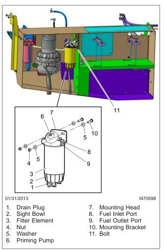
Fig. 3, Sidewall Mounted Fuel/Water Separator
