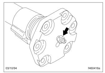
Fig. 90, Loosely Install the Sector-Shaft Adjusting Screw Jam Nut
