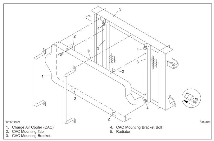
Fig. 1, Charge Air Cooler (CAC) Mounting
