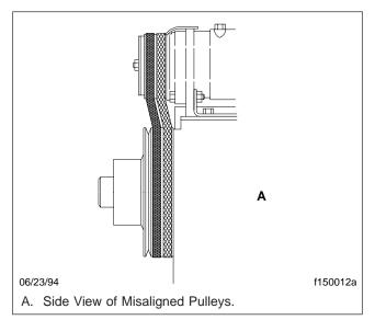
Fig. 3, Check for Misaligned Pulleys
