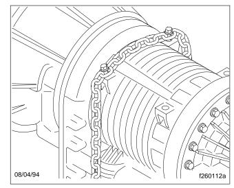
Fig. 6, Securing the Transmission With Chain
