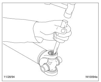
Fig. 1, Loosening the U-Joint Snap Ring
