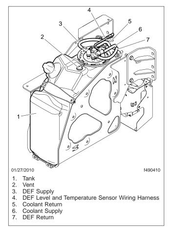
Fig. 1, DEF Tank and Header Unit Connections
