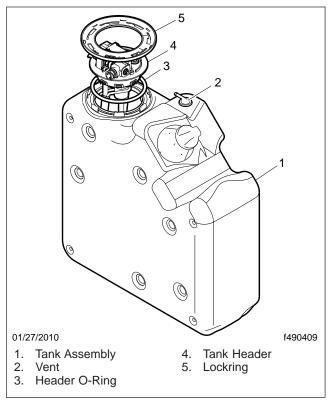
Fig. 2, Header Unit Assembly
