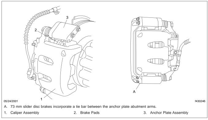
Fig. 2, Bosch Pin Slide Brakes Major Components
