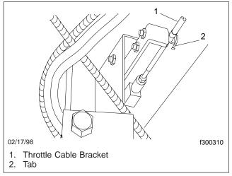
Fig. 1, Throttle Cable Bracket
