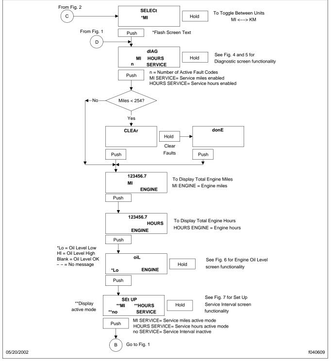
Fig. 3, Engine Miles and Service Interval Setup Screens
