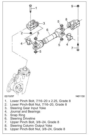
Fig. 1, Steering Driveline Installation
