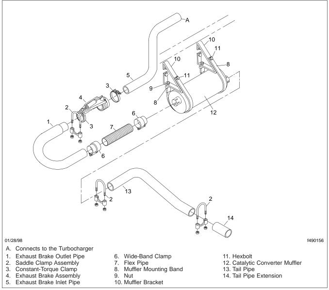
Fig. 1, Exhaust System Routing (rear-mounted engine, typical)
