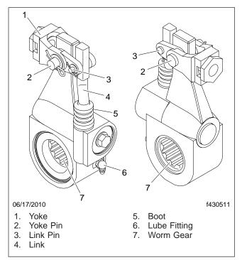
Fig. 1, ASA-5 Automatic Slack Adjuster
