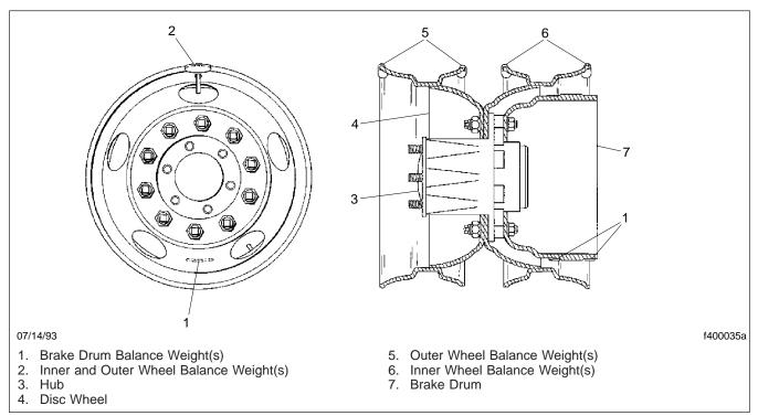
Fig. 1, Recommended Location of Wheel and Brake Drum Balance Weights
