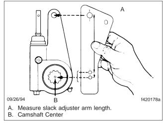
Fig. 5, Measure the New Slack Adjuster
