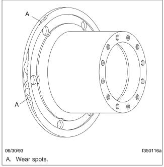
Fig. 1, Typical Wheel Hub, Damaged
