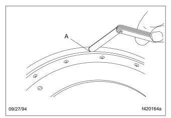
Fig. 4, Insert the Feeler Gauge between the Lining and Shoe Table
