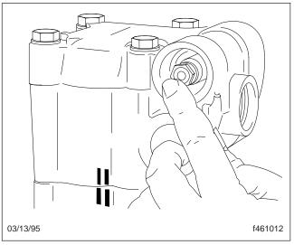
Fig. 37, Installing the Valve Spool Assembly
