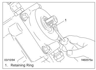
Fig. 3, Remove the Retaining Ring
