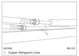
Fig. 3, Refrigerant Line Connections
