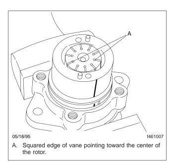
Fig. 32, Installing the Rotor and the Vanes
