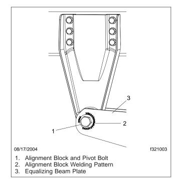
Fig. 1, Alignment Block Welded to the Equalizing Beam
