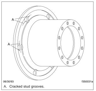
Fig. 2, Typical Wheel Hub, Damaged
