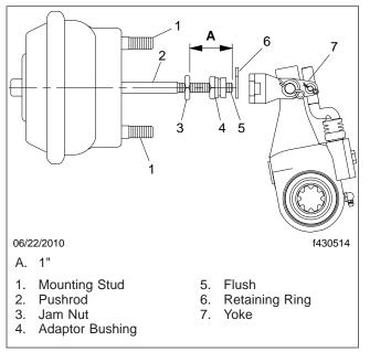
Fig. 4, Quick-Connect Yoke Assembly
