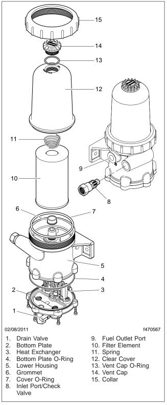
Fig. 1, Fuel/Water Separator (Fuel Pro 382 shown)
