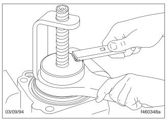
Fig. 26, Unscrew the Adjuster Locknut and Bearing Adjuster
