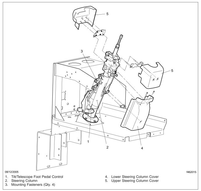
Fig. 1, Tilt/Telescope Steering Column Assembly
