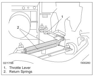
Fig. 1, Throttle Lever in Idle Position
