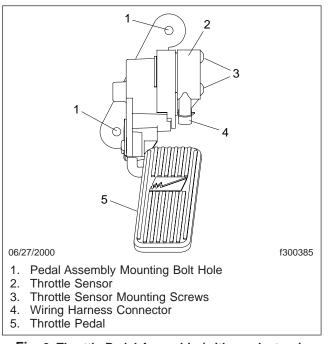
Fig. 3, Throttle Pedal Assembly (with an electronic automatic transmission)
