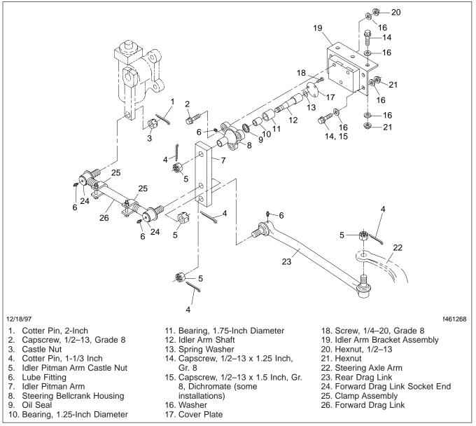
Fig. 1, Model XC Drag Link Assembly
