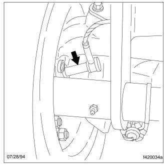
Fig. 1, Removing the Wheel Speed Sensor
