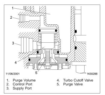
Fig. 4, AD-IP Turbo Cutoff
