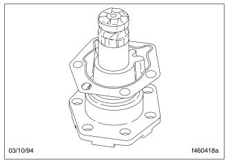
Fig. 92, Install the Side Cover Gasket
