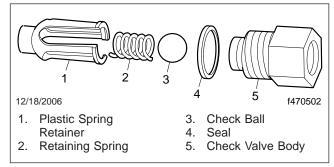
Fig. 3, Check Valve Assembly
