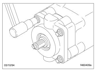
Fig. 83, Install the Valve Housing Bolts
