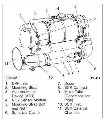
Fig. 1, Cummins Switchback ATD Installation
