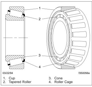
Fig. 2, Tapered Wheel Bearing Assembly
