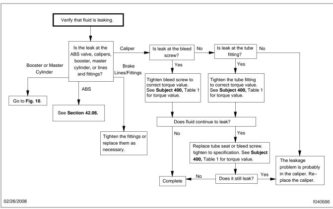
Fig. 9, Flow Chart: Hydraulic System Leakage
