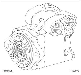
Fig. 1, TRW PS Series Power Steering Pump
