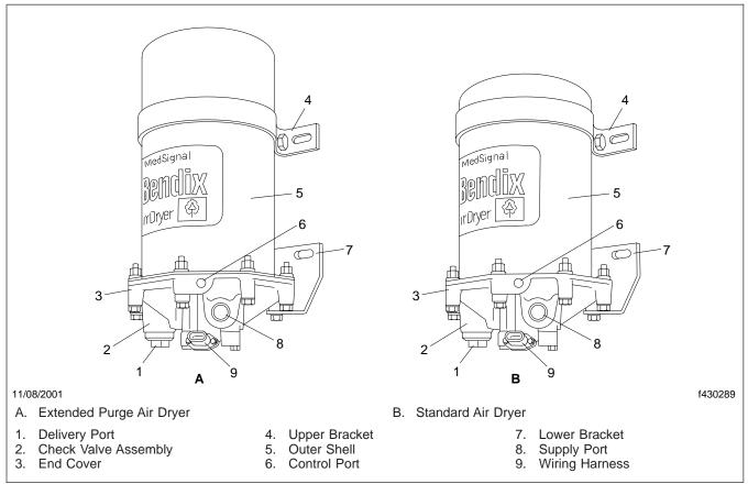
Fig. 1, Bendix AD-9 Air Dryer
