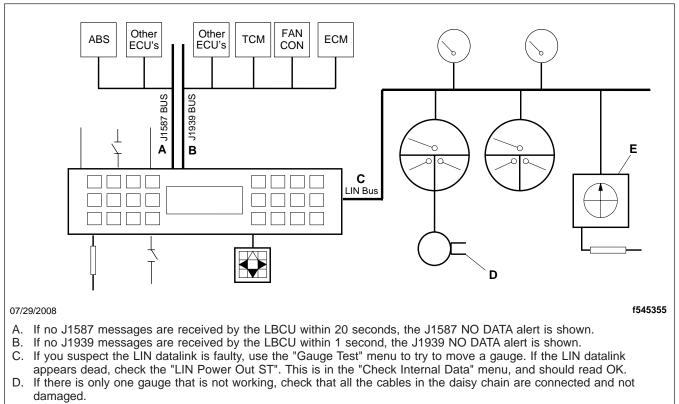
E. If the compass module is not properly connected or it is faulty, it will not show up in the menu. There is a 10 second time out before the compass line disappears due to loss of message on the LIN datalink line. If a message on either datalink is missing and there is no data received, the menu will show dashes for that data item (ROAD SPEED ------). When data driving a gauge is lost, the gauge will be sent to zero position.
