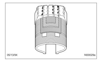
Fig. 2, Radial Ply Tire Construction
