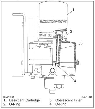
Fig. 1, Air Dryer (sectional view)
