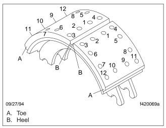
Fig. 3, Rivet or Bolt Attachment Sequence
