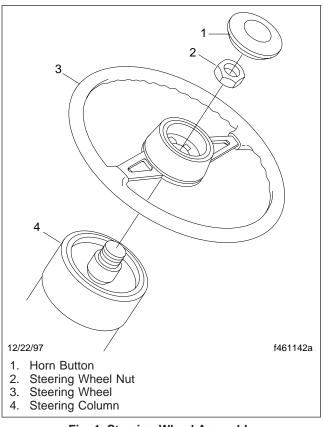
Fig. 1, Steering Wheel Assembly
