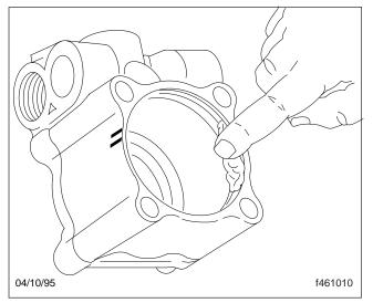
Fig. 35, Greasing the Sealing Areas
