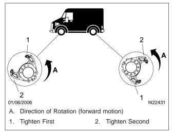
Fig. 6, Tightening Sequence for Caliper Mounting Bolts, Left Side
