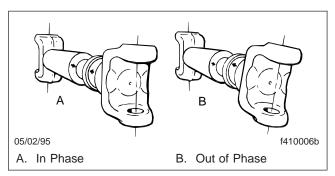
Fig. 2, U-Joint Phasing
