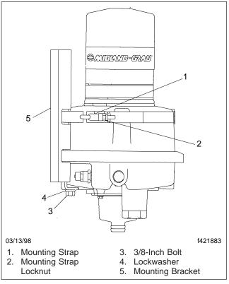
Fig. 1, Air Dryer Removal and Installation
