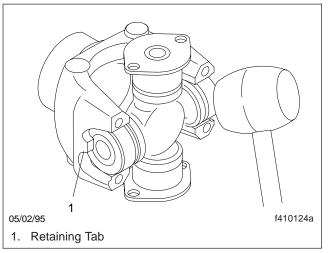
Fig. 4, Seating a U-Joint in a Half-Round End-Yoke
