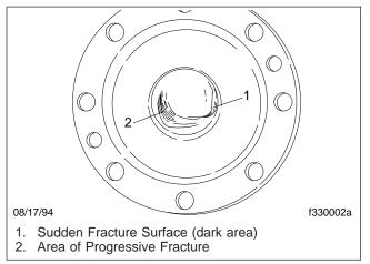
Fig. 7, Fatigue Fracture
