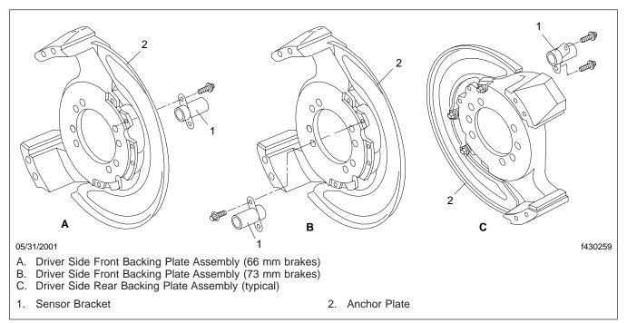
Fig. 3, Splash Shield and Sensor Mounting Bracket
