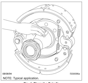
Fig. 4, Clean the Spindle
