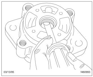
Fig. 17, Removing the Shaft Seal
