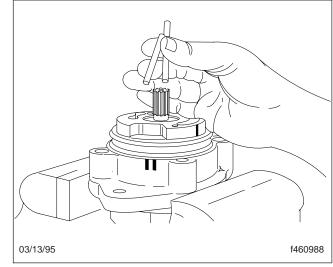
Fig. 12, Removing the Locating Pins
