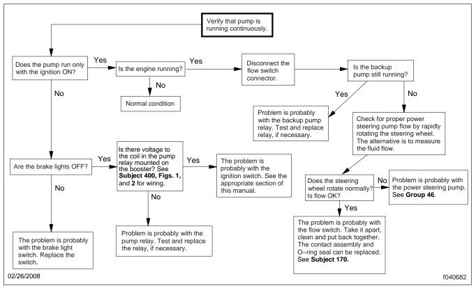
Fig. 3, Flow Chart: Backup Pump Runs Continuously
