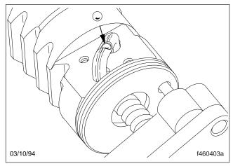
Fig. 77, Insert the Steel Balls
