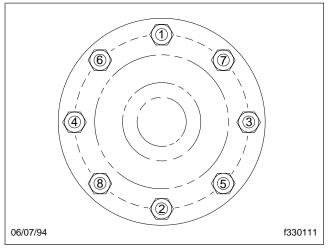
Fig. 10, Axle Shaft Flange Nut-Tightening Sequence
