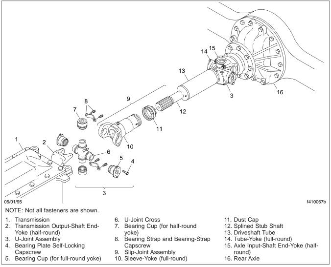
Fig. 1, Components of a Basic Driveline
