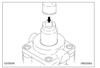
Fig. 32, Tap Out the Seal from the Valve Housing
