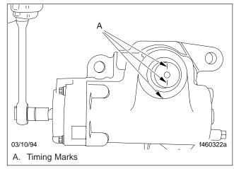
Fig. 104, Check the Timing Marks
