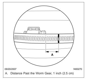
Fig. 2, Marking the Metal Strap
