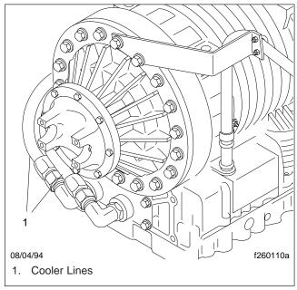
Fig. 3, ATF Cooler Lines
