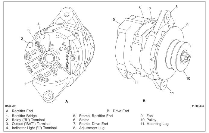
Fig. 1, 21-SI Alternator (exterior view)
