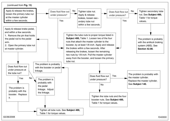
Fig. 14, Flow Chart: Brakes are Dragging (cont.)
