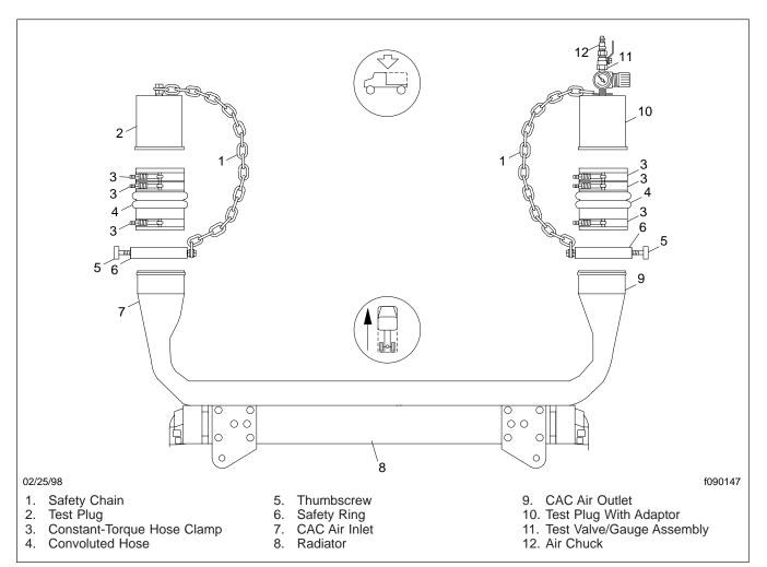
Fig. 1, CAC Core Leakage Test (rear-mounted CAC shown)
