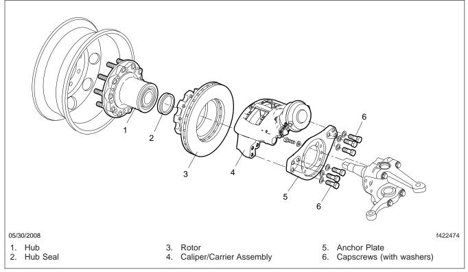
Fig. 1, Wheel End Assembly (exploded view)
