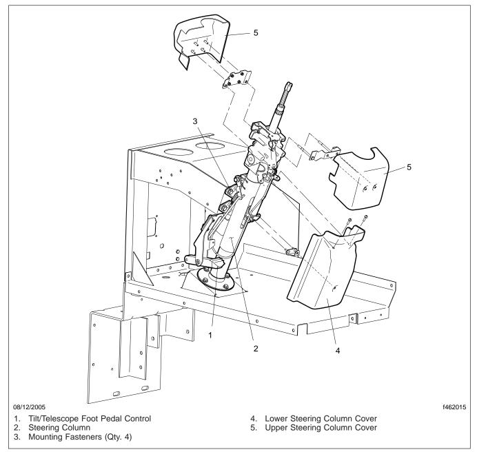
Fig. 1, Tilt/Telescope Steering Column Assembly
