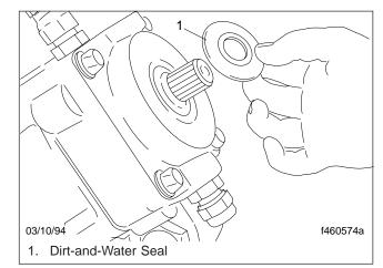
Fig. 2, Remove the Dirt-and-Water Seal
