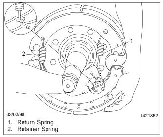
Fig. 5, Attach the New Brake Shoe Return Spring
