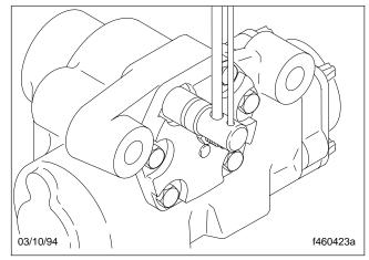
Fig. 98, Install the Special Side Cover Bolts
