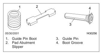
Fig. 5, Anchor Plate Components
