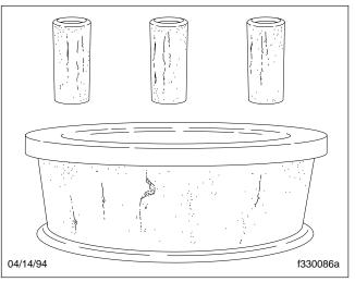
Fig. 9, Etching (Pitting) on Bearing Surfaces
