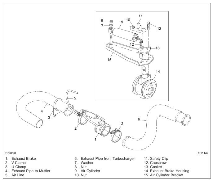
Fig. 3, Jacobs Exhaust Brake Installation
