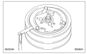
Fig. 10, Check the Clutch Clearance
