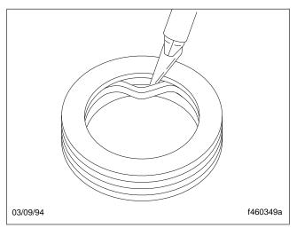
Fig. 27, Remove the Seal Ring and O-Ring
