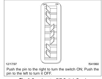
Fig. 2, Speedometer DIP Switch Panel
