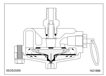
Fig. 3, Start of System Pressure Charging
