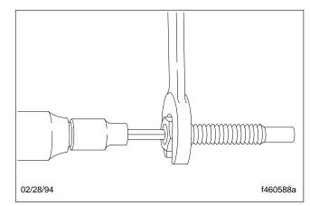
Fig. 3, Screw in the Poppet Adjusting Screw
