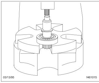
Fig. 26, Pressing the New Input Shaft
