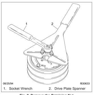
Fig. 2, Remove the Retaining Nut
