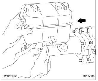
Fig. 4, Removing the Master Cylinder
