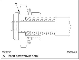
Fig. 3, Pull-Pawl Assembly (sectional view)
