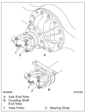
Fig. 8, Removing a Half-Round End-Yoke
