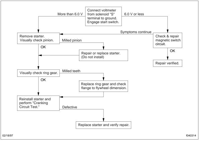
Fig. 1, Milled Pinion Symptoms
