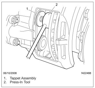
Fig. 3, On-Vehicle Installation of Tappet
