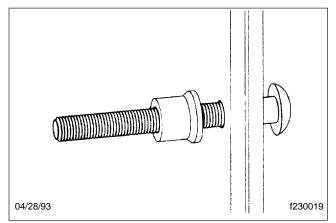
Fig. 5, Positioning the Collar
