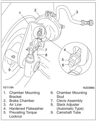
Fig. 1, Service Brake Chamber
