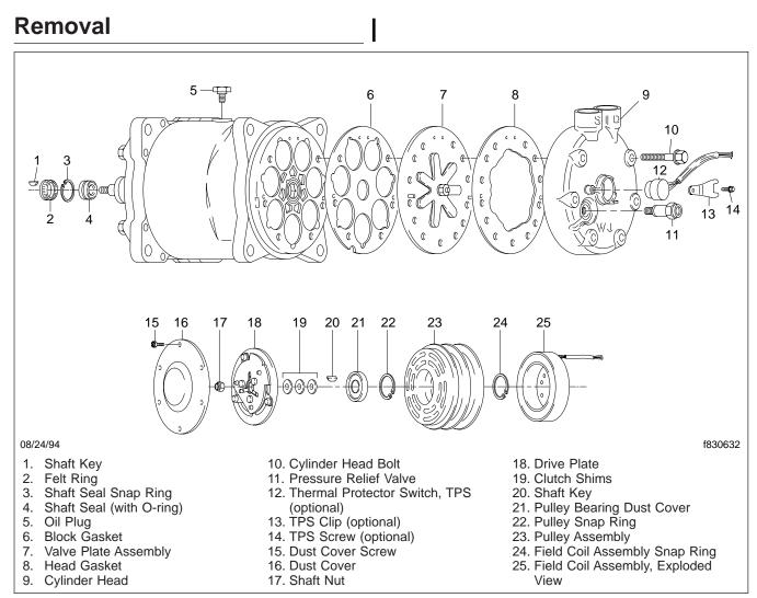
Fig. 1, Refrigerant Compressor, Exploded View
