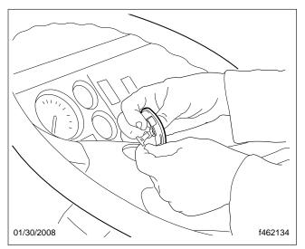
Fig. 1, Removing the Horn Button
