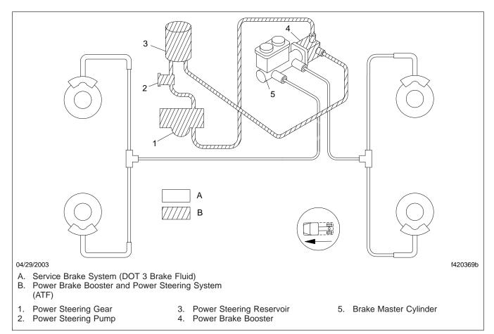
Fig. 2, Brake System Booster
