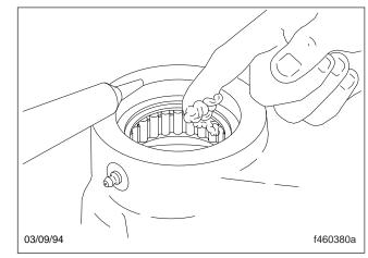
Fig. 55, Pack the Area between the Dirt Seal and the Pressure Seal with Grease
