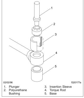
Fig. 2, Torque Rod Bushing Installation
