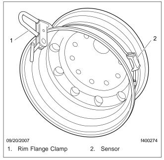
Fig. 4, Remounting Tires Using a Vertical Tire Machine
