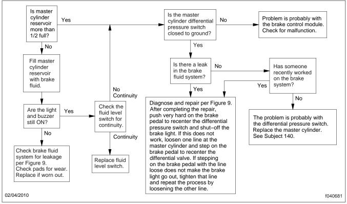
Fig. 2, Flow Chart: Brake Warning Lamp and Buzzer for Service Brake Problems
