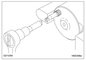
Fig. 72, Install a Poppet Adjuster Seat and Sleave Assembly
