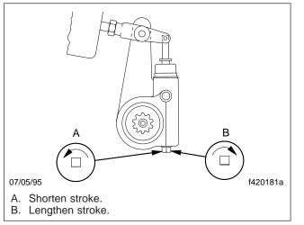
Fig. 11, Turn the Adjusting Nut
