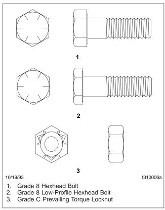
Fig. 6, Frame Fastener Identification
