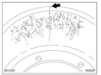
Fig. 4, Cracked Drums
