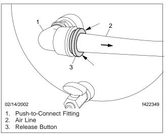
Fig. 4, Push on Release Button and Remove Air Line
