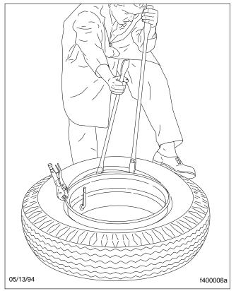
Fig. 6, Working the Upper Bead into the Rim
