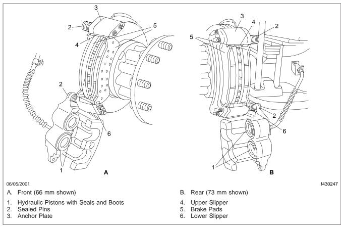
Fig. 3, Bosch Pin Slide Brakes System Components
