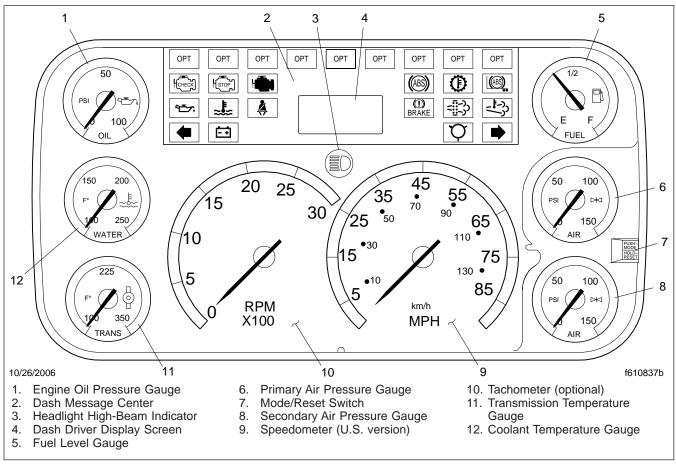
Fig. 1, Gauge Layout (typical, U.S.)
