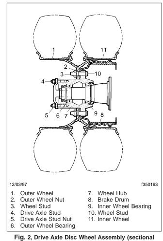
, Drive Axle Disc Wheel Assembly (sect view)
