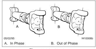
Fig. 6, U-Joint Phasing
