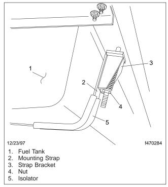
Fig. 1, Fuel Tank Mounting Strap Assembly
