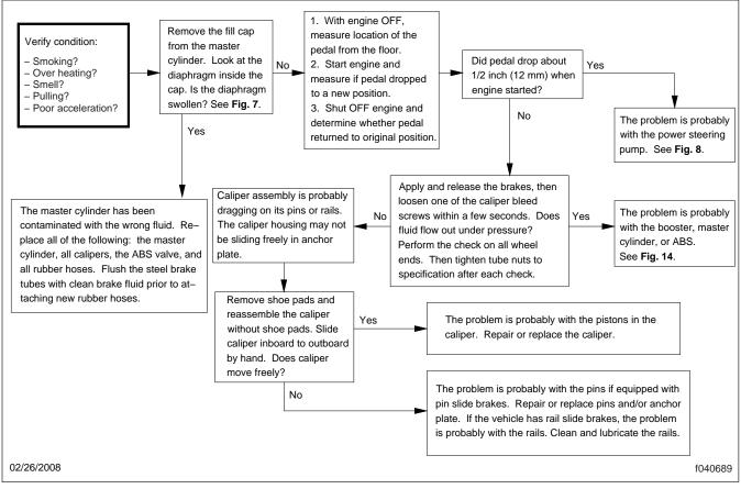
Fig. 13, Flow Chart: Brakes are Dragging
