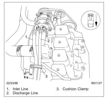
Fig. 1, Refrigerant Compressor
