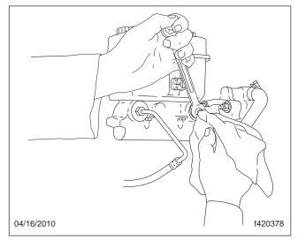
Fig. 2, Removing the Brake Lines
