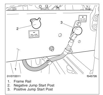
Fig. 1, Possible Jump Start Post Location (passengerside engine compartment)
