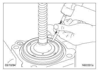
Fig. 65, Stake the Locknut to the Valve Housing and the Bearing Adjuster
