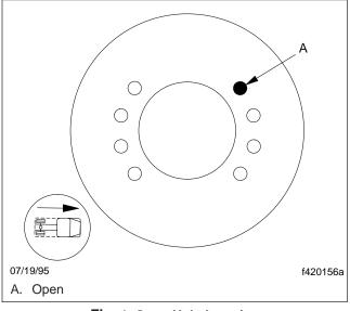
Fig. 1, Open Hole Location
