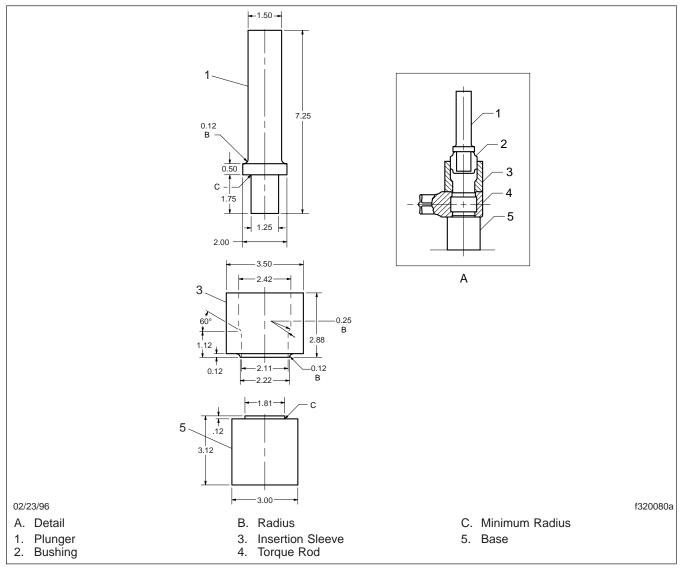
Fig. 1, Bushing Installation Tool
