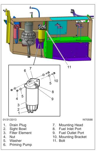
Fig. 3, Sidewall Mounted Fuel/Water Separator
