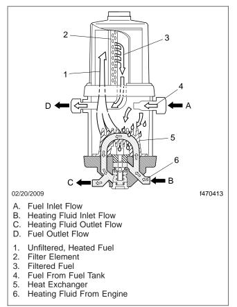
Fig. 5, DAVCO Fluid Circulation, Fluid-Heated Units
