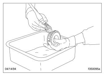
Fig. 8, Cleaning the Bearings
