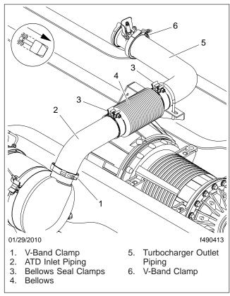
Fig. 1, Exhaust Piping, Engine to ATD
