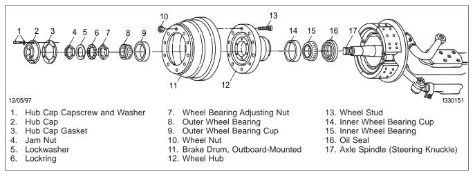
Fig. 1, Typical Front Axle (exploded view)
