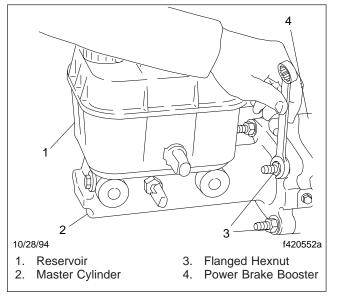
Fig. 3, Removing the Hexnuts
