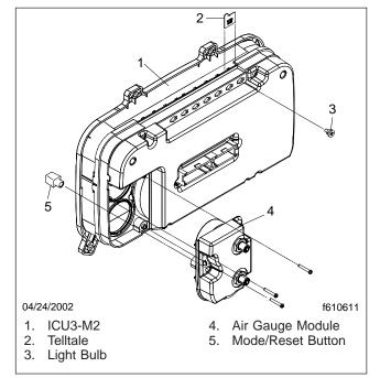
Fig. 2, ICU3-M2, Rear View (exploded)
