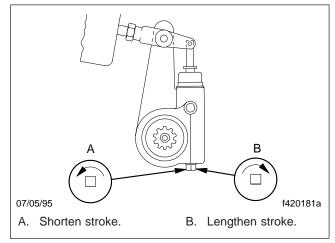
Fig. 8, Adjusting the Stroke
