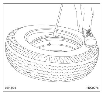
Fig. 5, Working the Lower Bead into the Rim
