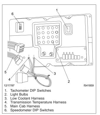
Fig. 1, Back of Instrument Cluster
