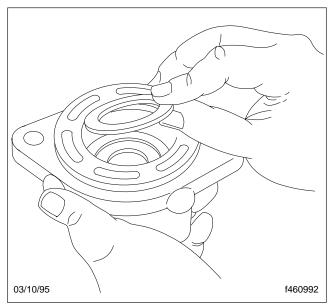
Fig. 16, Removing the Spacer
