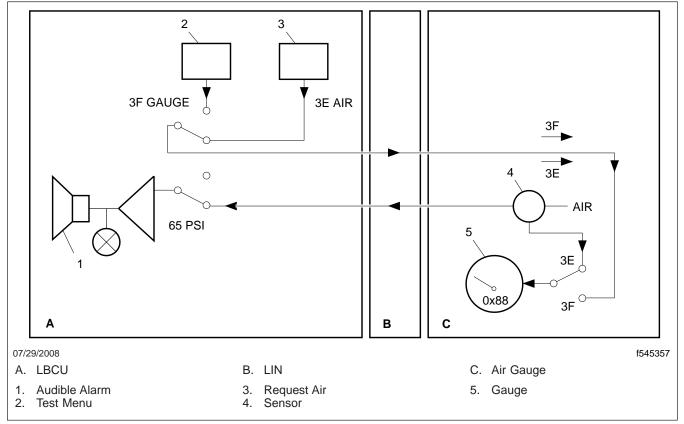
Fig. 6, Air Pressure Message on LIN
