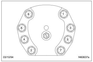
Fig. 97, Eight-Bolt Tightening Sequence
