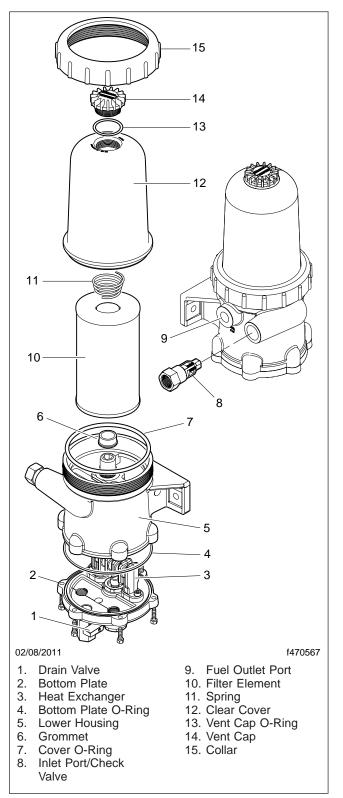
Fig. 1, Fuel/Water Separator (Fuel Pro 382 shown)
