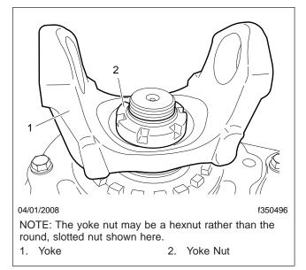
Fig. 1, Yoke Nut on the Carrier
