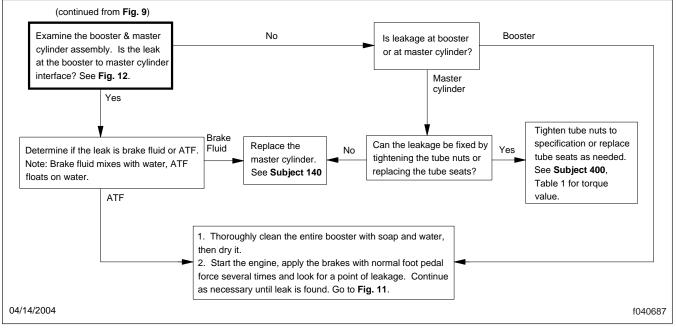
Fig. 10, Flow Chart: Hydraulic System Leakage (cont.)
