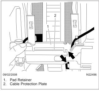
Fig. 2, Electronic Wear Indicator
