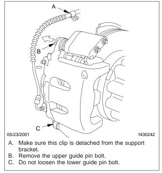
Fig. 3, Caliper Upper Guide Pin Bolt Removal
