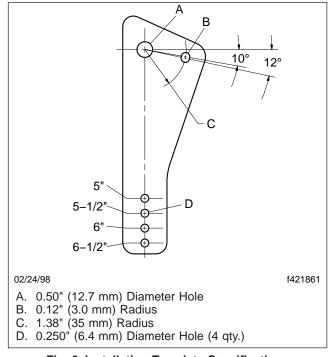
Fig. 6, Installation Template Specifications
