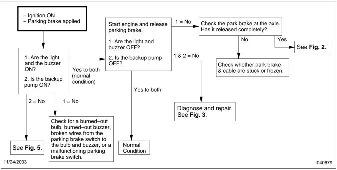
Fig. 1, Flow Chart: Brake Warning Lamp and Buzzer Relating to Parking Brake
