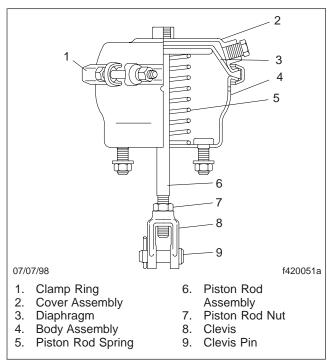
Fig. 1, Brake Chamber (sectional view)
