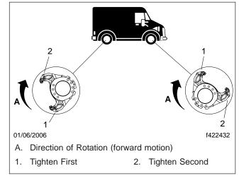
Fig. 7, Tightening Sequence for Caliper Mounting Bolts, Right Side
