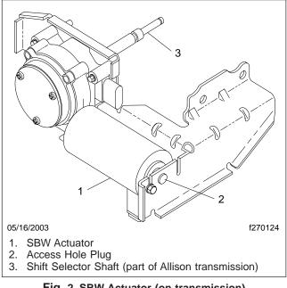
Fig. 2, SBW Actuator (on transmission)
