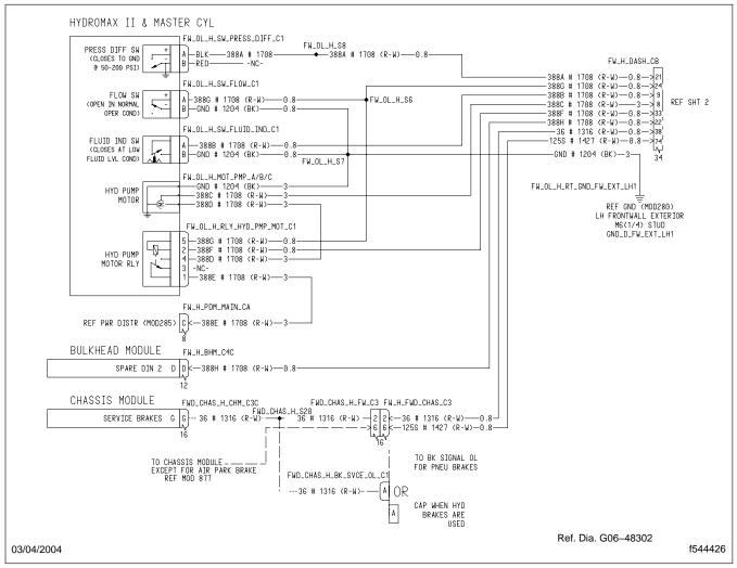
Fig. 1, Hydraulic Brake Frontwall Wiring
