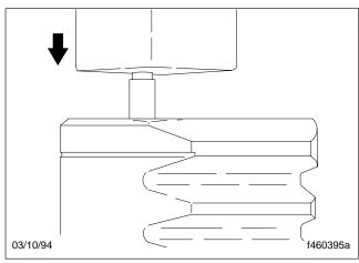
Fig. 69, Press the Adjuster Seat Into the Adjuster Sleeve
