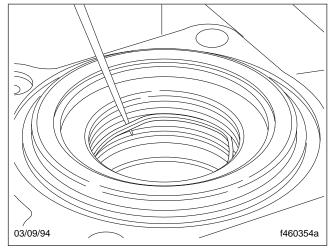
Fig. 30, Remove and Discard the Seal Rings and O-Rings from the Valve Housing
