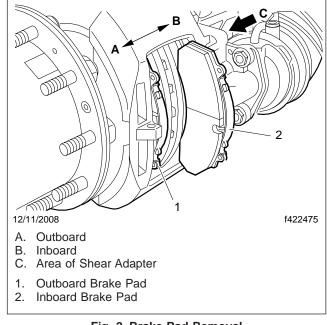
Fig. 2, Brake Pad Removal
