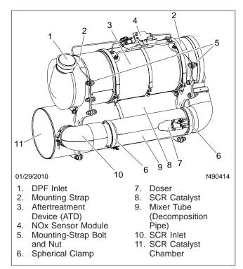
Fig. 1, Cummins SCR Catalyst Installation
