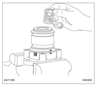
Fig. 7, Removing the Spring
