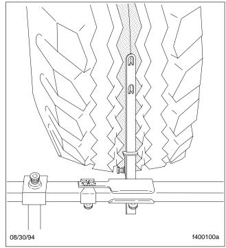
Fig. 3, Calculating Wheel Toe-In
