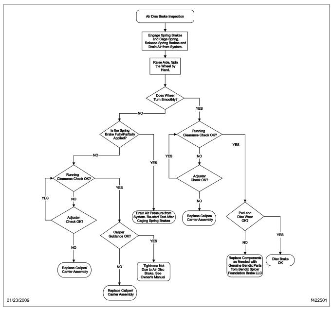
Fig. 1, Bendix Air Disc Brakes Troubleshooting Flowchart
