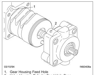
2. Valve Housing Cylinder Feed-Hole Boss
