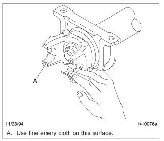
Fig. 12, Smoothing a Half-Round End-Yoke Cross-Hole
