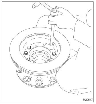
Fig. 1, Rotor-to-Hub Fasteners
