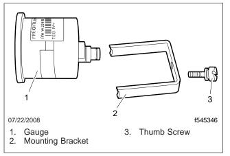
Fig. 2, Thumb Screw Mounted Gauge
