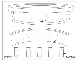
Fig. 7, Indentations, Cracks, or Breaks in Bearing Surfaces
