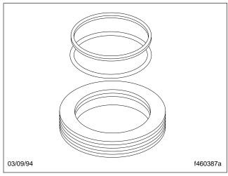
Fig. 61, Lubricate the New O-Ring and Seal Ring
