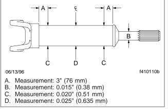
Fig. 2, Used Driveshaft Runout Specifications
