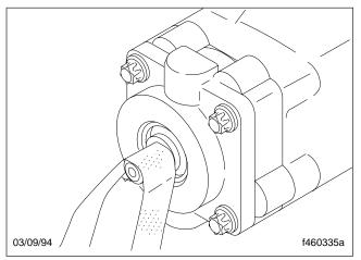
Fig. 13, Clean the Input Shaft
