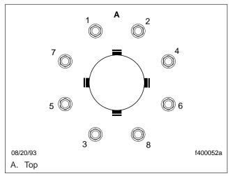
Fig. 1, 8-Stud Disc Wheel Tightening Sequence
