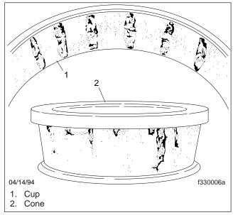
Fig. 3, Spalling (Flaking) of Wheel Bearing Assembly
