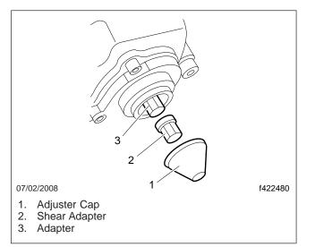
Fig. 3, Shear Adapter
