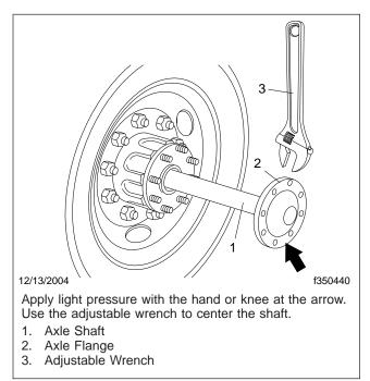
Fig. 1, Installing the Axle Shaft
