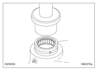
Fig. 50, Press the Roller Bearing into the Housing
