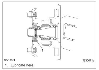
Fig. 8, Lubricate the Bearings
