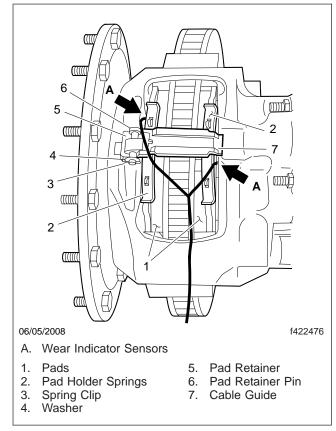
Fig. 1, Electronic Wear Indicator
