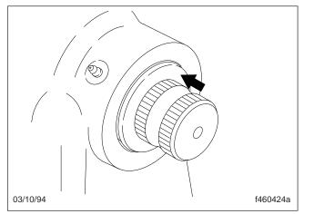
Fig. 99, Install a New Trunnion Dirt Seal
