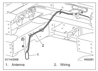
Fig. 1, TPMS Wiring From the Antenna
