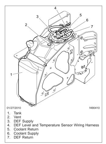
Fig. 1, 13-Gallon Tank Ports
