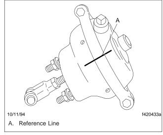
Fig. 2, Marking a Reference Line
