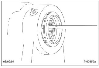
Fig. 35, Remove the Dirt Seal
