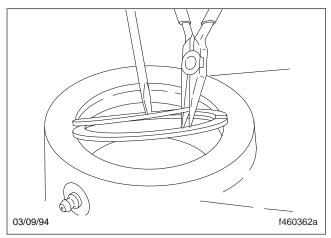
Fig. 38, Remove the Retaining Ring
