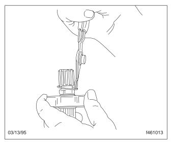
Fig. 24, Removing the Retaining Ring
