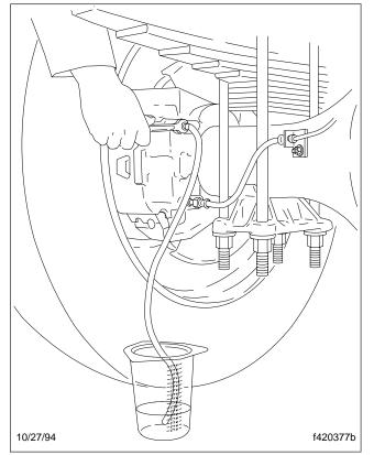
Fig. 2, Bleeding the Connections at the Rear Wheel Calipers First.
