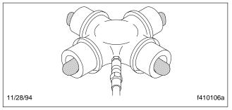
Fig. 14, Forcing Out Old Lubricant From a U-Joint Cross
