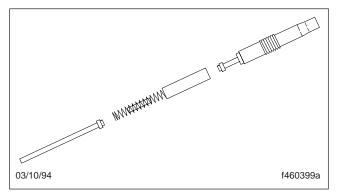
Fig. 73, Install the Poppet Assembly Parts
