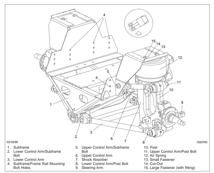
Fig. 1, Front Suspension Assembly (three-quarter view from rear)
