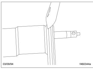
Fig. 21, Cut the Teflon Seal Ring
