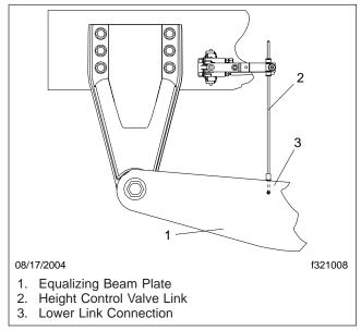
Fig. 1, Height Control Valve Linkage
