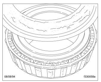
Fig. 9, Bearing Damage Resulting from Inadequate Lubrication
