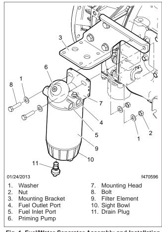
Fig. 1, Fuel/Water Separator Assembly and Installation
