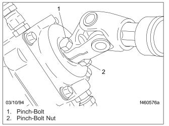
Fig. 4, Install the Pinch Bolt
