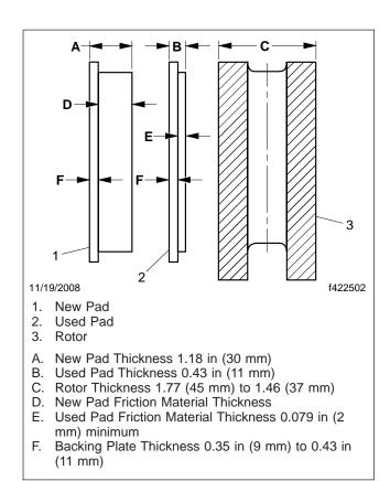
Fig. 5, Brake Pad Inspection
