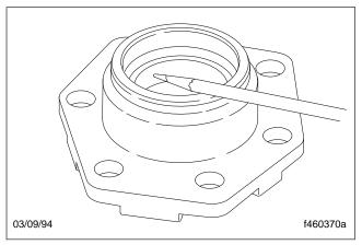
Fig. 46, Inspect the Side Cover Bushing
