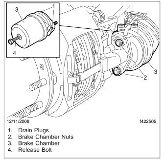
Fig. 2, Service Brake Chamber
