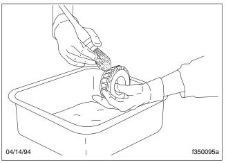
Fig. 5, Wheel Bearing Cleaning
