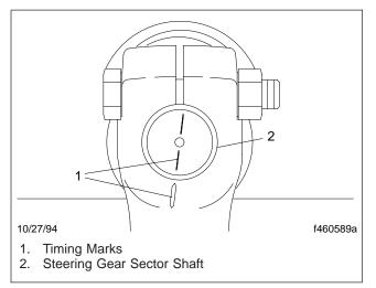
Fig. 2, Position the Pitman Arm on the Steering Gear
