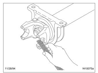
Fig. 11, Removing Burrs From a Half-Round End-Yoke Cross-Hole
