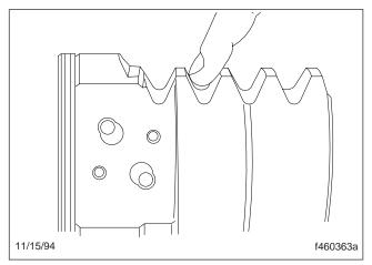
Fig. 39, Inspect the Rack Piston Teeth
