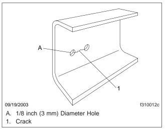
Fig. 1, Preventing Cracks from Spreading
