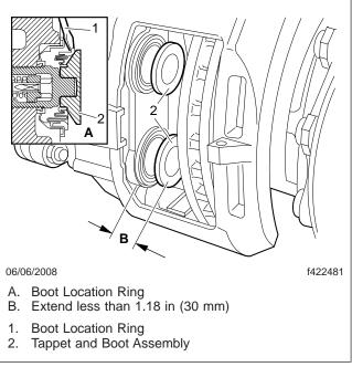
Fig. 4, Tappet and Boot Assembly
