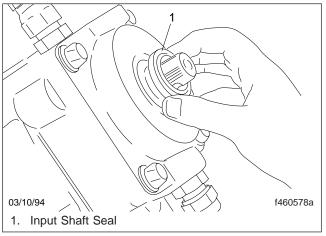
Fig. 6, Install the Input Shaft Seal
