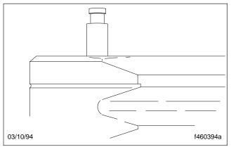
Fig. 68, Adjuster Seat/Adjuster Sleeve in the Rack Piston
