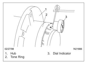
Fig. 3, Positioning the Dial Indicator
