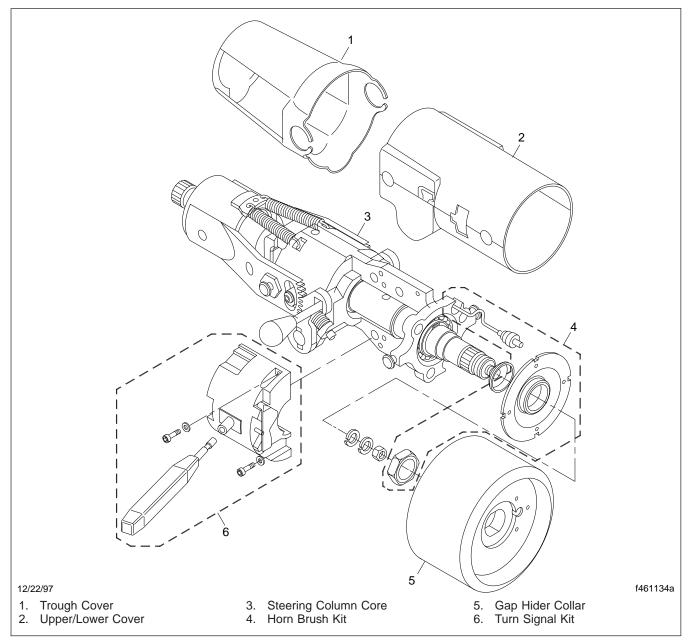
Fig. 1, Tilt Steering Column Assembly
