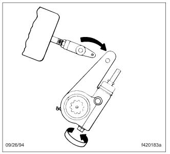
Fig. 4, Move the Slack Adjuster Away from the Clevis
