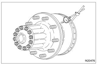
Fig. 2, Measuring Runout
