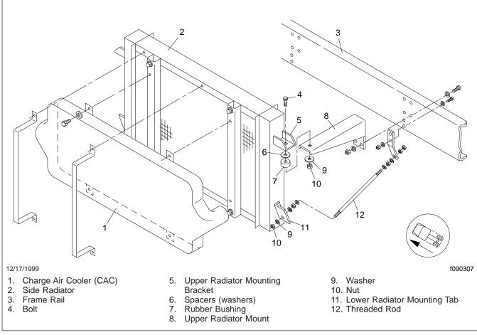
Fig. 4, Side Radiator Mounting
