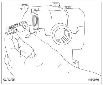
Fig. 3, Removing the Spring
