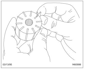
Fig. 22, Checking the Vanes
