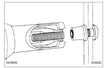
Fig. 8, Installed Huckbolt Fastener
