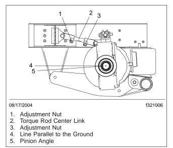
Fig. 1, Pinion Angle Adjustment
