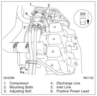
Fig. 1, Refrigerant Compressor
