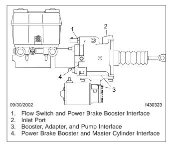
Fig. 12, Potential Hydraulic Fluid Leak Points
