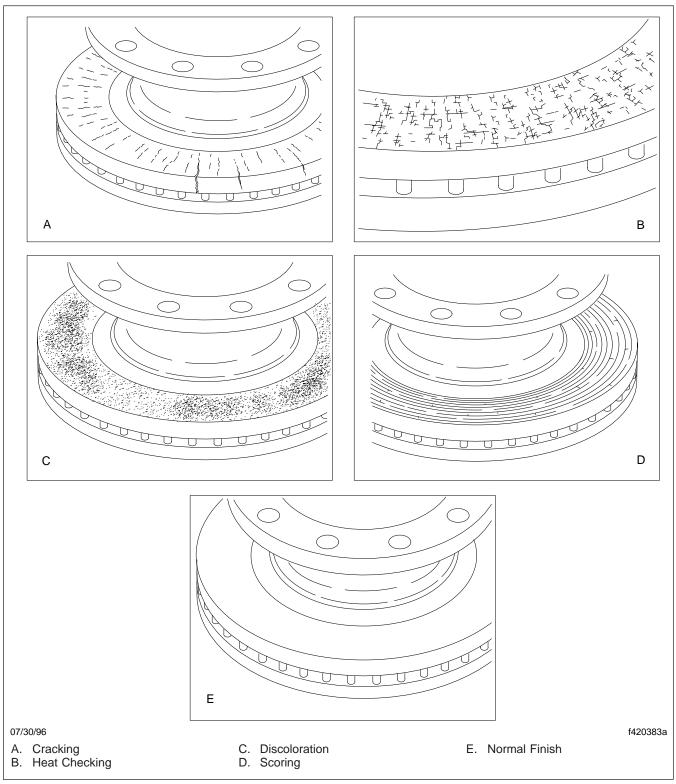
Fig. 2, Rotor Surface Check
