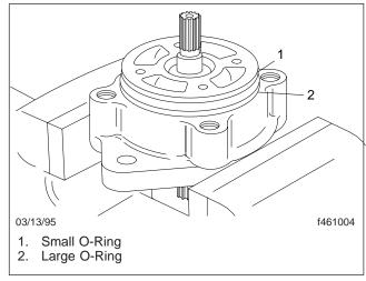
Fig. 29, Installing the O-Rings
