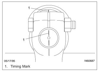
Fig. 1, Position the Sector Shaft
