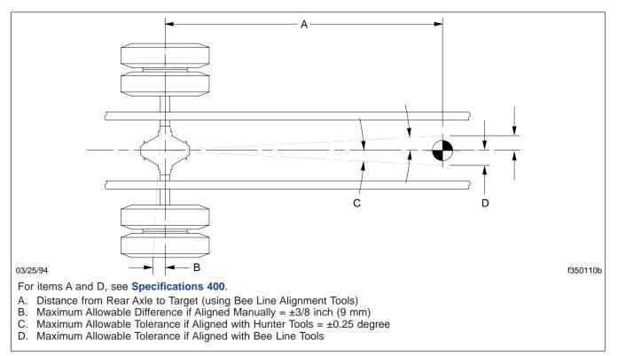
Fig. 1, Alignment Measurements
