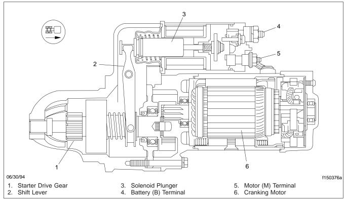
Fig. 2, Starter Components
