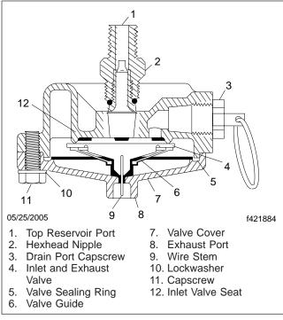
Fig. 1, DV-2 Valve (cutaway view)
