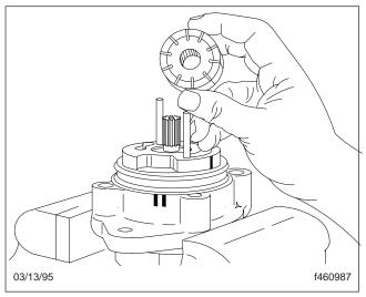
Fig. 11, Removing the Rotor and Vanes
