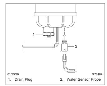
Fig. 1, Water Sensor Probe
