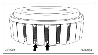
Fig. 11, Rubbing Marks on Bearing Cage
