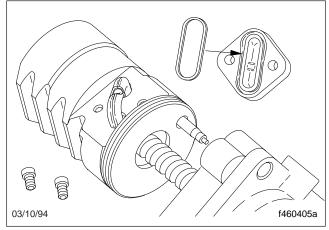
Fig. 79, Install the Seal
