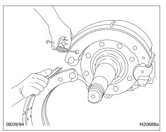
Fig. 4, Attach the New Springs
