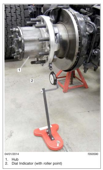
Fig. 2, Setup to Measure Radial Runout
