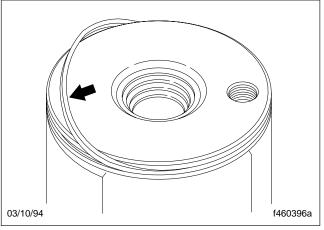
Fig. 70, Install a new Backup O-Ring and new Teflon Seal Ring
