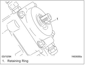
Fig. 101, Install a New Retaining Ring
