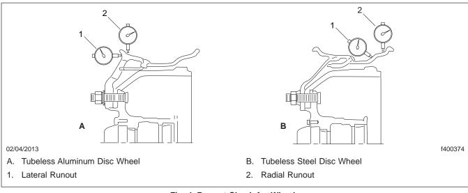
Fig. 4, Runout Check for Wheels
