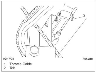
Fig. 1, Throttle Cable Bracket
