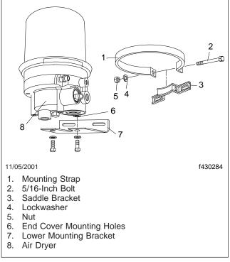
Fig. 1, Bendix AD-IP Air Dryer
