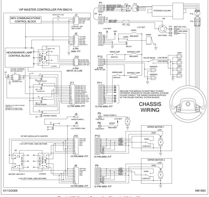
Fig. 1, VIP Master Controller Chassis Wiring Diagram
