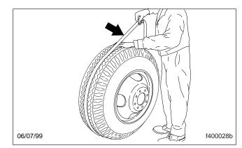
Fig. 4, Endless Pi Tape
