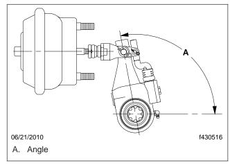
Fig. 5, Installation Angle
