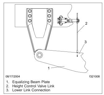
Fig. 2, Height Control Valve Linkage
