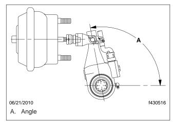
Fig. 1, Installation Angle
