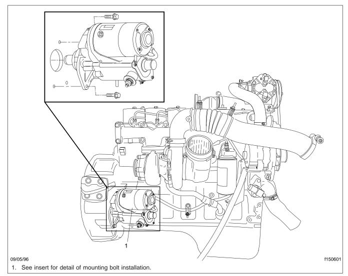
Fig. 3, Starter Installation
