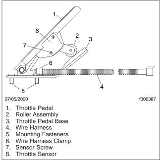
Fig. 2, Felsted Electronic Throttle Pedal (right-side view)
