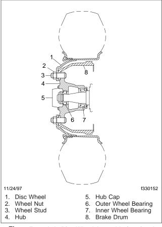
Fig. 1, Front Axle Disc Wheel Assembly (sectional view)
