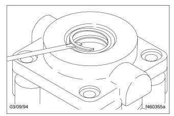
Fig. 31, Remove the Retaining Ring
