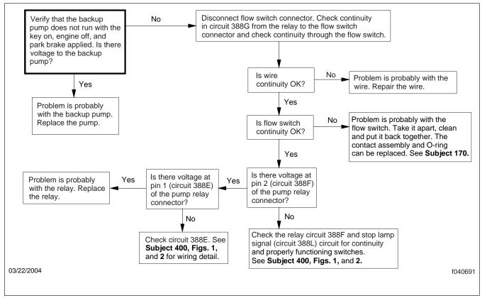
Fig. 5, Flow Chart: Backup Pump Does Not Run
