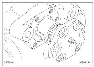
Fig. 95, Install the Sector Shaft and Side Cover
