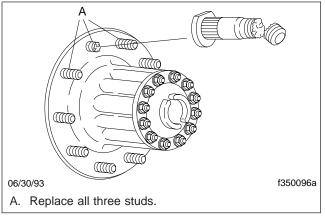
Fig. 1, Replacing Damaged Studs
