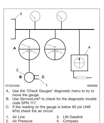
Fig. 5, Air Pressure Gauge Check
