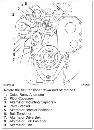
Fig. 3, Alternator Installation, Cummins B Series Engine
