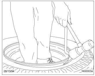
Fig. 1, Loosening the Beads
