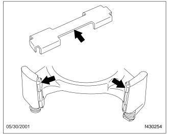
Fig. 7, Pad Abutment Slipper
