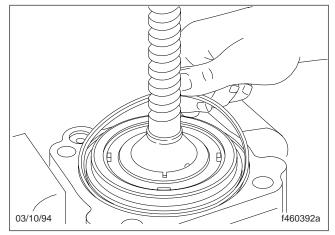
Fig. 66, Install the New Grease Seal Rings
