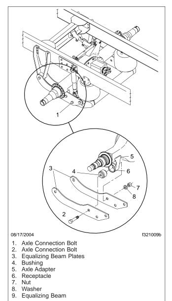
Fig. 2, Axle Adapter Bushing Replacement
