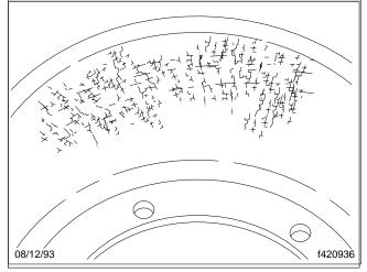
Fig. 3, Heat Checking
