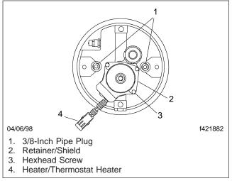
Fig. 1, Purge Valve Replacement
