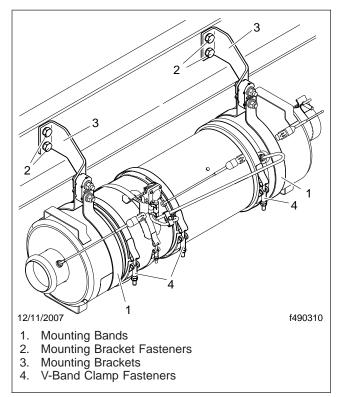
Fig. 2, Aftertreatment Device Mounting
