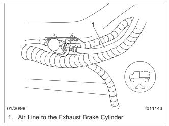
Fig. 1, Disconnecting the Exhaust Brake Air Line
