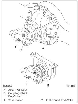
Fig. 9, Removing a Full-Round End-Yoke
