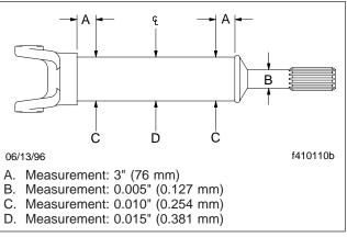
Fig. 18, Driveshaft Runout Specifications
