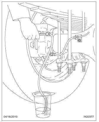
Fig. 2, Bleeding the Hydraulic Connection
