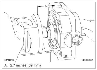
Fig. 78, Check the Valve Housing Pilot Face
