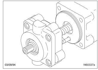
Fig. 15, Remove the Valve Housing
