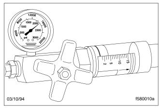
Fig. 3, Power Steering System Analyzer
