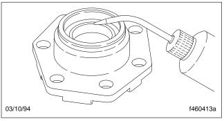
Fig. 87, Applying Oil to the DU Bushing
