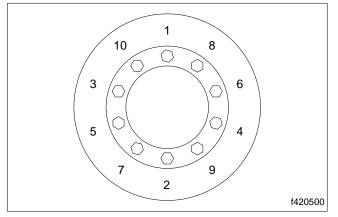
Fig. 4, Tightening Pattern
