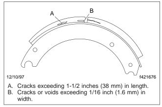
Fig. 1, Cracks and Voids
