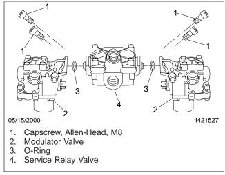
Fig. 1, Modulator Valve Assembly
