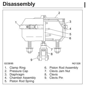
Fig. 1, Brake Chamber (sectional view)
