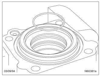
Fig. 56, Lubricate and Install a New O-Ring
