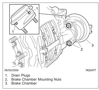
Fig. 1, Service Brake Chamber Installation
