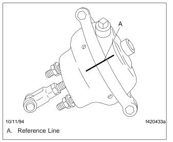
Fig. 2, Marking a Reference Line
